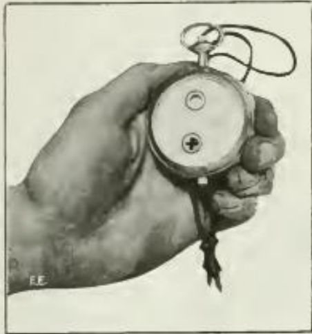
A Watch Style Polarity Indicator of the Magnetic Type Appeals to Every Electrical Man. Details for Making One Are Given Herein.
