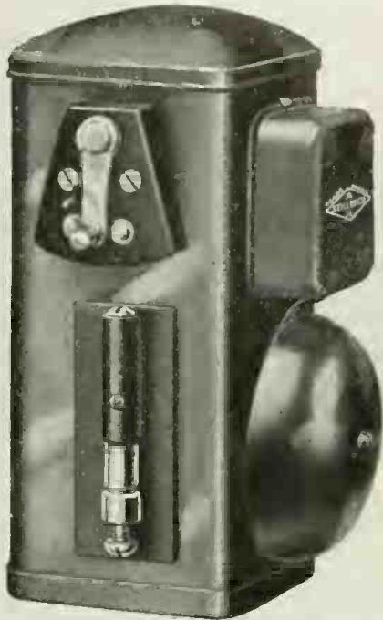
An Electric Fire Detector Which Can Be Left at Any Point Desired. Such as in the Kitchen, and as Soon as Blaze Occurs the Alarm Bell Rings. It Utilizes a Fine Mercury Column, Which Expands When Heated, Thus Closing the Bell Circuit. It Will Also Announce a Drop in Temperature.
