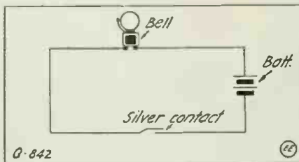
A Simple Yet Difficult Problem. It Is Required to Break This Circuit With a Minimum of Sparking and the Interrupter Is a Delicately Mounted One, Easily Vibrating With a Slight Jar.
