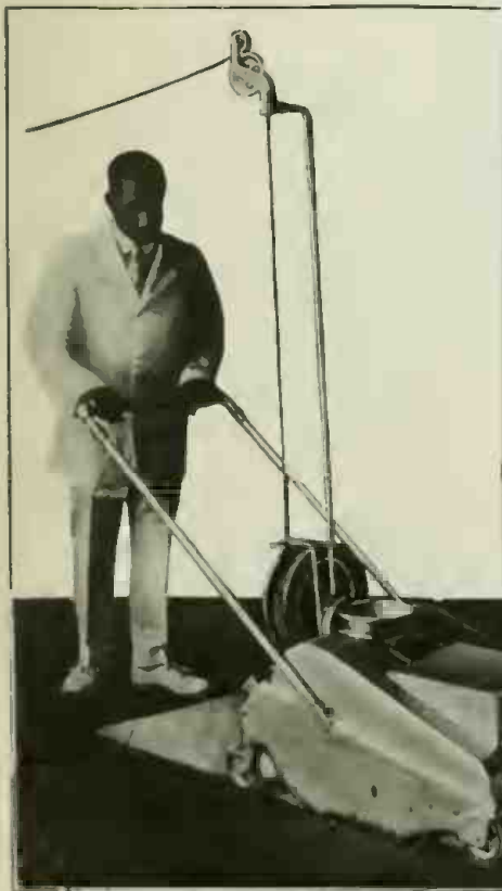
A 1/4 H.P. Electric Scrubbing Machine for Use in Large Buildings and Halls. It Reels Up or Unreels Its Electric Supply Cable as It Goes Along.
