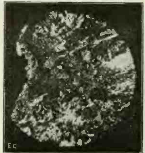
Fig. 2. Anode End Showing Where the Terminal Burnt Off. After the Silver Plating Was Destroyed by the Sulfur, the Outcropping of Silver Took Place. Magnified 50 Diameters.
