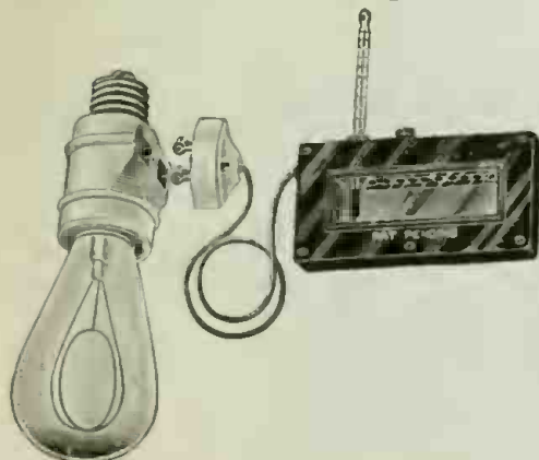
Fig. 7. This Miniature Electric Incubator for Microscope Stages Enables the Physician to Study "Live" Bacteria Organisms.
