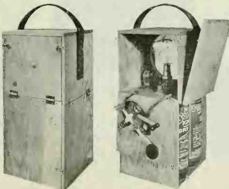
A Military Signal Projector Having a Range of 25 Miles. It is Fitted with 5-in. Mangin Mirror and 6-Volt 12-c.p. Mazda Lamp. A Telegraph Key Controls the Lamp Circuit.
