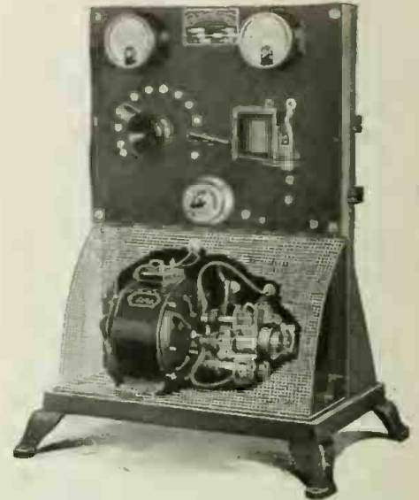
One of the Jobs We All Hate to Tackle is Charging Storage Batteries. In This Simple Automatic Device a Motor Drives a Commutator in Such a Way that the Alternate + and - A. C. Pulses Are All Rectified or Converted Into Direct Current.
