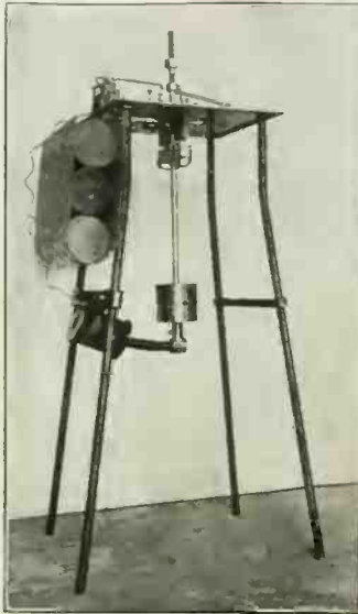
In Connection with Some Research Work in Aerodynamics Need Arose for an Instrument that Would Close a Battery Circuit at One Second Intervals, the Apparatus Shown Having Fulfilled the Requirements Very Satisfactorily. As a Test It Was Run for 24 Hours with a Deviation of a Few Seconds Only.
