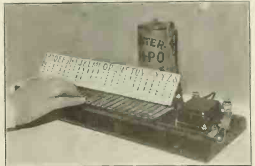
The "Simplograph"—An Attempt to Make the Learning of the Telegraph Code as Simple as Possible. A Buzzer Sounds the Signals for Radio Students.
