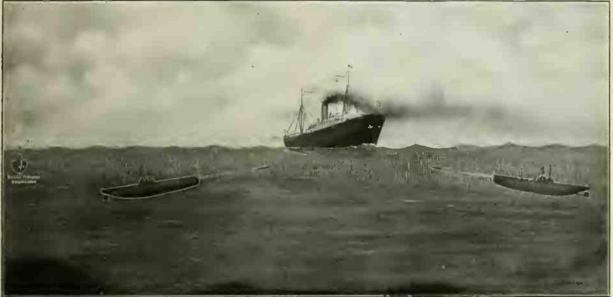
The Latest Reports Regarding Submarine Activities Frequently State that the Ship Was Torpedoed by an "Unseen" Sub-sea War-vessel. This Can Easily Be True for, by Utilizing Telegraphic Sound-waves Propagated Thru Water (Fessenden System), a Relatively Distant "Range-finding" Submarine Can Signal Her Hidden Allies as to the Position and Course of the Enemy. Thus the Submarine That Fires the Fatal Torpedo Need Never Show Its Periscope.
