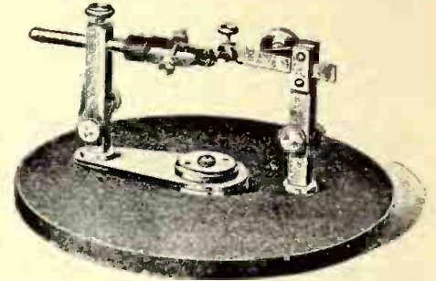
Carborundum Detector with Clamp Mounted on Rotatable Arm.
