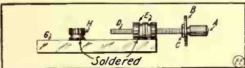
Micrometer for Measuring Wire, Made of 32-Pitch Screw and Nuts.
