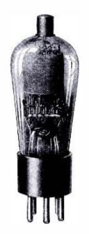
the special cathode construction, the heater voltage may vary during the charge and discharge cycles of the automobile storage battery, without affecting seriously the performance or serviceableness of this tube. No resistor in the heater circuit is required for operation from a six volt battery.
