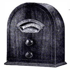
This converter is known as the Rembert and is illustrated above. The manufacturers claim that it will receive police calls, ship to shore, short wave phones and all short wave stations from 15 to 200 meters.
