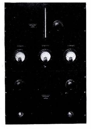
tions on the same channel, as beat note interference is reduced to a minimum and the range of the stations materially increased. To utilize this accuracy a means has been provided to shift the frequency over a few cycles to obtain zero beat for isochronous operation. This adjustment once made with a station having equally good frequency regulation, needs only an occasional check to maintain such operation.
