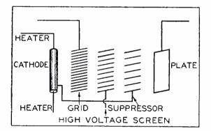
Above illustration gives a pictorial diagram of the arrangement of the elements in the new 239 type super-control tube. Tentative characteristics will be found on page 42
