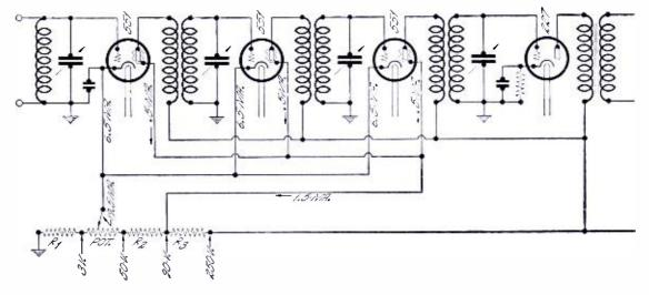
even though the correct ratios are maintained, a wide choice of resistance values was possible. Usually the current in the entire bleeder determines this factor. The current should be great enough so that the variation due to the volume control change will not lead to a serious change in other voltages. Let us start by using a 5000 ohm potentiometer for the volume control. If we calculate the current for a drop of 50-3 or
