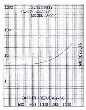
noninductive load resistance of 7000 ohms was connected across the plate circuit of the single 247 pentode output tube, which in turn was capacitatively coupled to the output indicating tube voltmeter, which read the standard audio level of .05 watts, except for power overload measurements. To prevent its impedance reflection on the plate circuit of the output tube, the voice coil circuit was disconnected during measurements.
