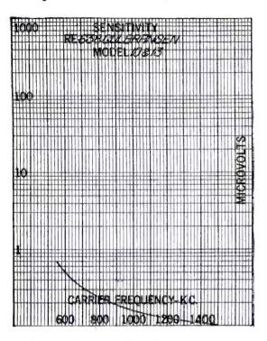
cuit was through the dummy antenna standard of 20 uh, 200 uuf and 25 ohms, while the receiver output was maintained at the standard audio level of .05 watts. A non-inductive load resistance of 7000 ohms matched the operating impedence of the single 247 output tube employed. The plate was capacitatively coupled to the output indicating tube voltmeter, and to avoid the loading effect of the voice coil on the primary of the speaker transformer, the secondary circuit was broken.
