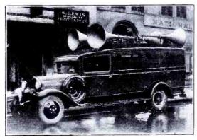
events, etc., where large crowds are gathered. A picture shows a Graybar Western Electric public address truck in which there is installed a Universal Electric Plant to run the amplifying equipment. Mr. R. C. Mulnix, Denver, Colorado, owner of this truck, recently completed a successful tour to handle the sound amplification for various public events in Colorado, Montana and Wyoming.
