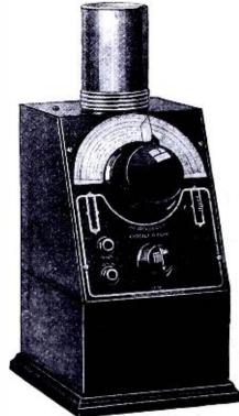
The manufacturer states that this instrument produces fundamental frequencies from 115 to 280 kc and harmonics from 230 to 1680 kc and higher. This equals approximately 175 to 2600 meters. The tuning dial is operated by a slow motion non-backlash vernier with a ratio of 68 to 1, permitting the setting of the dial pointer to hair line accuracy.
