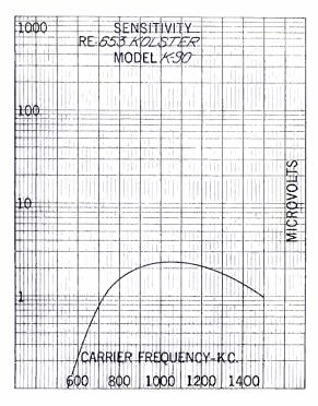
output through the receiver input circuit. The plate circuit of the pushpull power pentodes was matched with a non-inductive resistance load of 14,-000 ohms, while the voice coil was disconnected to prevent the reflection of its impedance on the primary circuit. A standard output of .05 watts of audio power was maintained with the output indicating device capacitatively coupled to the plates of the output tubes.
