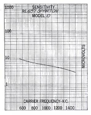
and the plate of the output power pentode was capacitatively coupled to the output indicating voltmeter, which read the voltage corresponding to a standard output of .05 watts, except for the power overload data. A noninductive resistance load of 7000 ohms was connected in the output circuit of the 247 pentode to match its operating impedance load.
