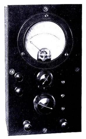
the value specified as 43,000 ohms, for which a 50,000 ohm unit was employed. To adjust this resistor the terminal at one end was loosened and moved along until, with a 45 volt battery, the terminals marked X shorted, and the rheostat set to about its middle position, the meter read just full scale, i. e., zero ohms.-
