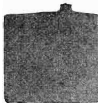
Fig. 2. A positive plate ready for use
