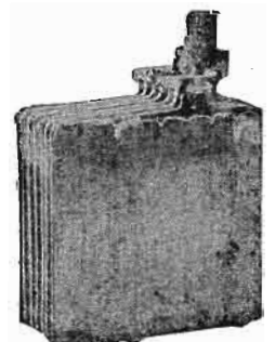
Fig. 4. Group showing excessive sulphation on plate due to lack of water
