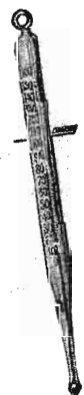
Fig. 12. Shows a temperature thermometer for a storage cell with the maximum heat at 110 degree, safe operating temperature
