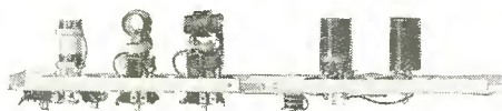
Fig. 9. This photograph shows the intermediate section before being placed in the chassis. Each of the I. F. coils has its respective padding condensers
