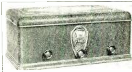
Fig. 2. There are only two controls on the panel of the receiver as shown in this photograph. The one at the left is for volume and regeneration while the center control is that of the tandem tuning condenser. The on-off switch is located at the right. The cabinet is of metal and serves as a shield for the receiver
