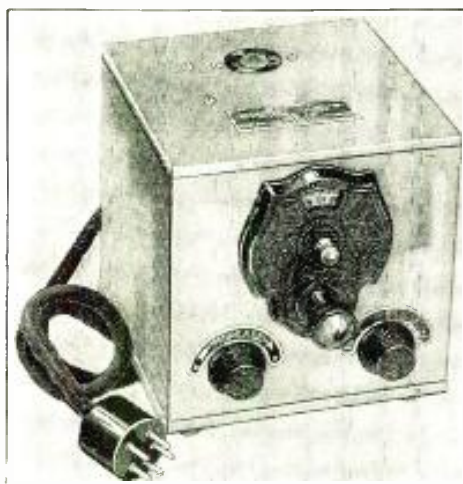
Fig. 1. This is the first model of the Scott short wave converter described for the first time in the accompanying article
