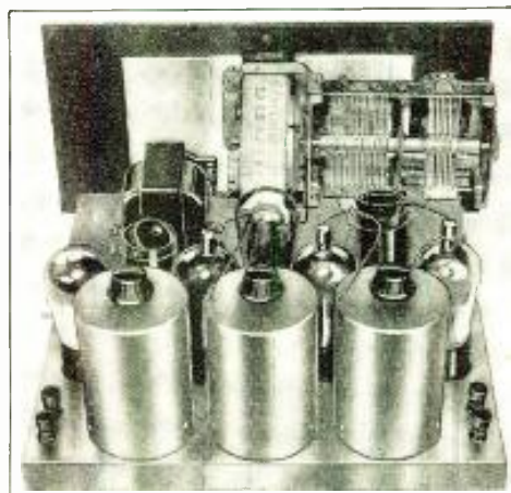
Fig. 2. Model B shown here is an a. c. superheterodyne screen grid tuner for use with a standard power amplifier
