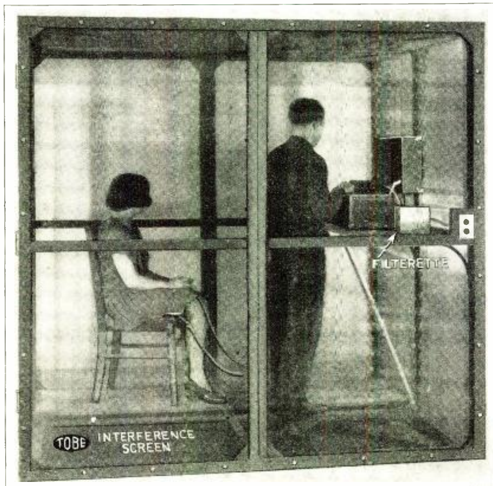
Fig. 1. Here is shown an interference screen placed around the apparatus with the patient and the operator inside
