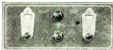
Fig. 2. The front panel arrangement of the Pilot short wave receiver is illustrated above
