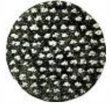
Fig. 7. A magnified portion of a threaded rubber insulator, showing the cotton threads
