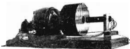
Fig. 3. This photograph shows the motor, drum scanner and the neon tube, the latter going in the center of the drum. This Jenkins scanner is now being used by several experimenters in picking up signals from 3XK at Washington, D. C.
