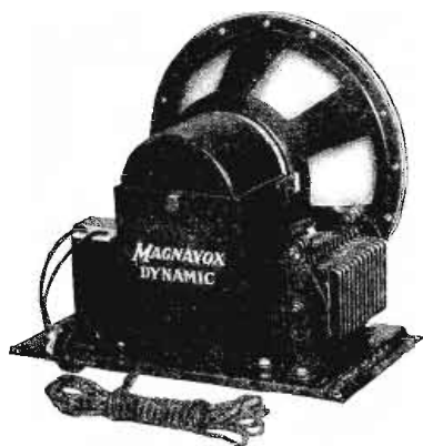
Fig. 2. This illustration shows the Magnavox dynamic operated from a.c. and available either in the 25 cycle or 60 cycle models. The rectifier is shown at the right of the unit
