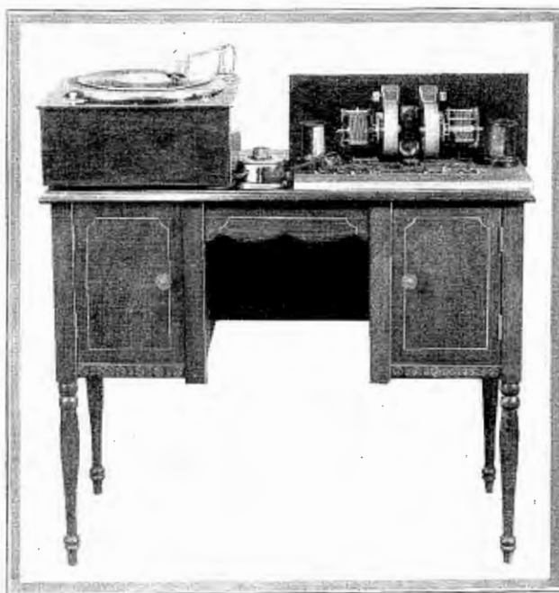
Figure 6. With a standard record pickup and record turntable the set may be used for radio or record reproduction with good tone
