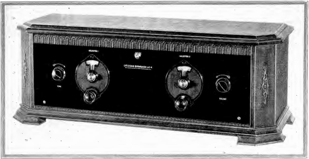
Figure 2. Placed in a Corbett cabinet, the Citizens Birnbach A. C. Four is illustrated above
