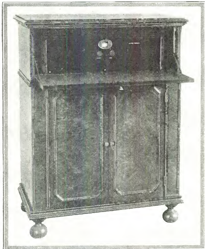
Figure 4. Here the Unitune Symphonic may be seen placed in an Excello console. Suitable A and B supplies may be placed inside the console if so desired
