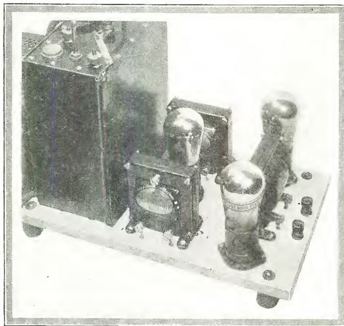
Figure 5. This photograph represents the push-pull audio amplifier end of the eliminator, whose connections are represented in the schematic circuit Figure 7 on this page
