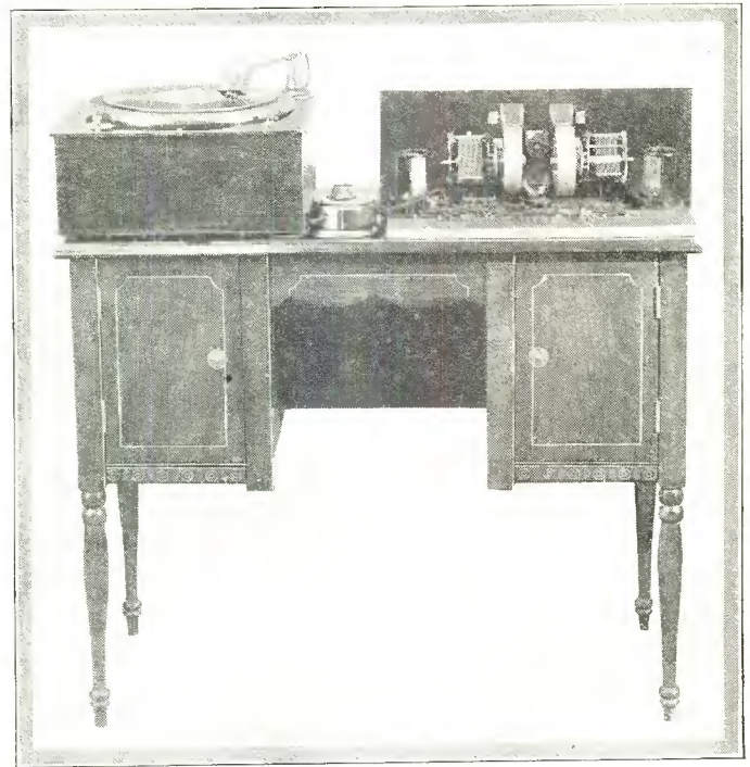
Figure 5. In this photograph may be seen an electric phonograph with its electrical pick-up, while at the right is shown a rear view of the S-M Universal tuner. The console table is a Southern Toy product
