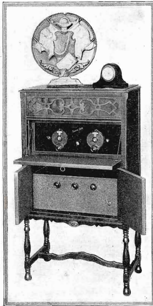
Photo A. View showing receiver and complete power amplifier installed in a console
