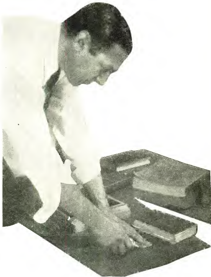
Figure 3. In making the G. R. P. speaker the back cone is weighted. With one finger preventing the cement from seeping between the cones, apply the Ambroid cement around the circumference of the back cone
