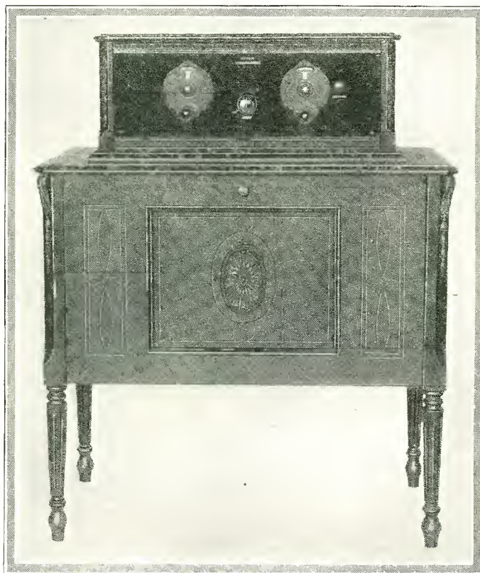
Figure 1. This photographic view shows the National Browning-Drake amplifier placed in a cabinet and located on top of an artistic table. If desired, the power amplifier which goes with the set may be placed inside of the table, since room is not provided on top
