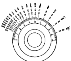
Stations partially separated and tuning slightly improved with a Straight Line Wave Length Condenser.
