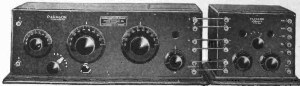
Type RD-5 Regenerative Receiver (including Detector)
