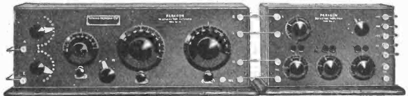
Type RA10—Regenerative Receiver. Type DA2—Detector Amplifier.
