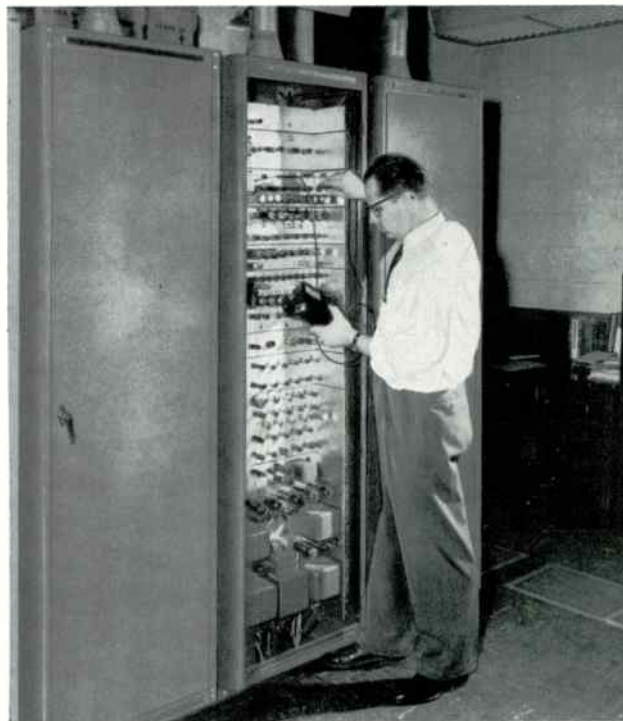
Above, the Phonevision sound coder. Scrambling the picture alone is not sufficient. Sound must be scrambled also to prevent unauthorized reception by a non-subscriber.
