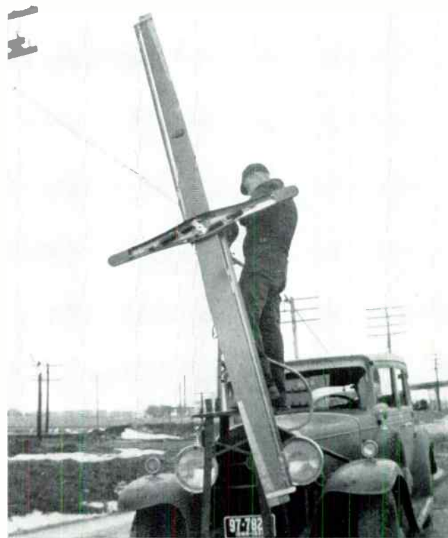
Early Wincharger development work used on automobile instead of wind tunnels for testing.
