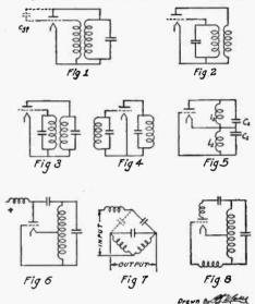
On shorter wavelengths, however, electrostatic couplings between the coils and the tube elements become very important and at very high frequencies may exceed the magnetic coupling. Care must therefore, be taken in the layout for high frequencies as the capacitive and inductive couplings are usually of opposite sign.
