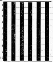
The scanning beam in this example thus travels across one line in 1-100 of a second. Inasmuch as it takes one complete change from a dark to a light area (or the opposite) to create one cycle of current in the photo electric cell, then for
