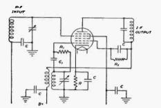
These tubes when built into a circuit must be thoroughly shielded; the capacity in the output or plate circuit of this tube should be large enough to limit the output voltage built up across this circuit in order to prevent degenerative effects. It should be at least 50uuf.
