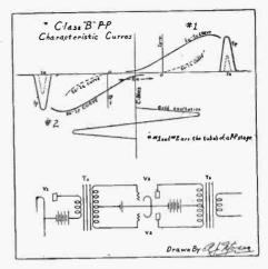
grids are excited, as shown below, a pulse of plate current flows for alternate half cycles, in the plate circuit of each tube. Since these pulses of plate current of each tube do not flow during the same half cycle each current will set up a strong D. C. field necessitating the use of a large core for Te in order to minimize the possibility of core saturation.
