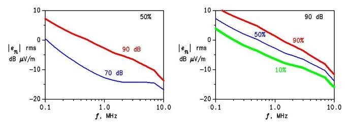
Figure 6. Variation of atmospheric-noise levels with frequency
