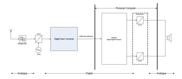
Figure 4 Block diagram of a DDC-based receiver.
