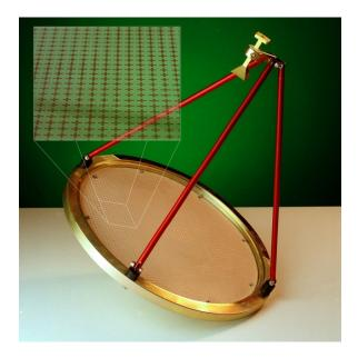
Figure 8. Circularly polarization reflectarray (20 GHz).
