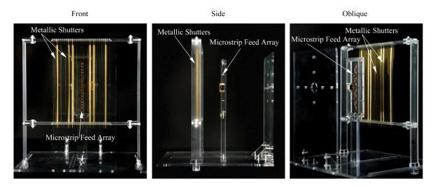
Figure 13. Fresnel zone plate shutter antenna with beam scanning capability.
