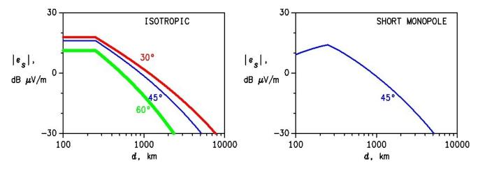
Figure 9. Median MF sky-wave signal strength.
