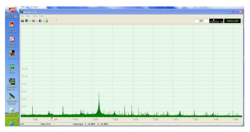
Figure 1 An SDR-view of the 1.8MHz CW band, using the band scope in VE3NEA's *Rocky* application software and a SoftRock v6 receiver, viewed on the screen of VK6VZ's Pentium IV personal computer. The signals you can see were recorded around local sunrise during the CQ 160 CW contest on 21 January 2006. The x axis of the band scope shows the frequency in kHz, whilst the y axis shows the amplitude of the signal in dB.
