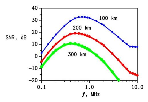
Figure 8. Ground-wave signal-to-noise ratio.
