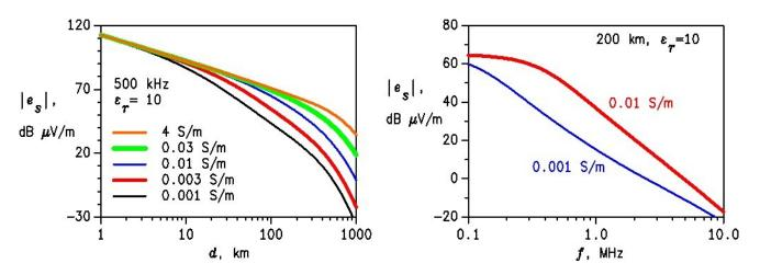
Figure 7. Amplitude of the ground-wave signal.
