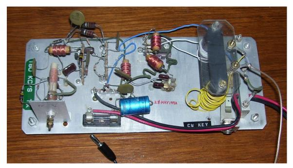
Figure 1 180 kHz Transmitter
