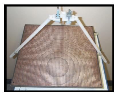
Figure 7. Dual-polarization bifocal reflectarray (20/30 GHz).
