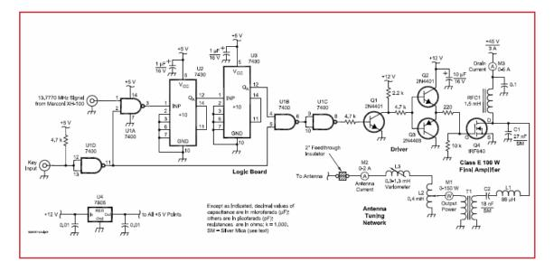
*Figure 3* 137 kHz transmitter schematic. From July 2005 QST, reprinted with permission. Copyright ARRL.
