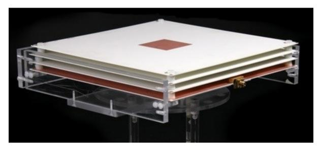
Figure 5. Stacked patch for wideband L-Band mobile satellite communications.
