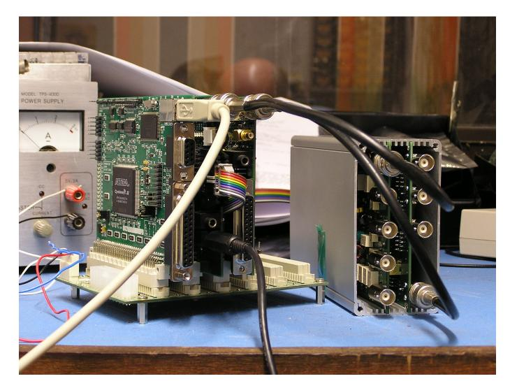
Figure 5 Photo of VK6APH's prototype transceiver. On the left (from left to right) you can see the Ozy, Mercury and Pentelope boards. On the right are prototype ALEX receiver bandpass filter and transmitter low pass filter, boards mounted in case.
