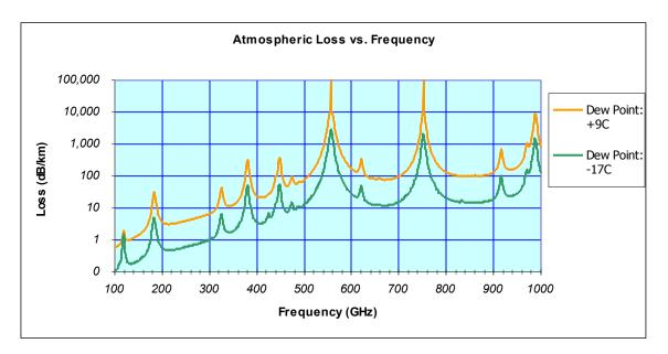
This graph shows the total atmospheric losses from both water vapor and oxygen as a function of operating frequency. When one locates the amateur millimeter wave bands on the graph (122, 134 & 241 GHz) it can be seen that there distinct advantages to operating at those frequencies due in-part to their distance from fixed molecular line resonances such as 119 and 183 GHz. This becomes even more of an issue when one considers operation in
