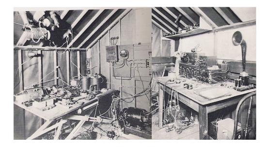
**Figure 3** Picture on the left, the 1BCG transmitter, employing four type "P" Radiotron UV204 vacuum tubes, the oscillator tube on the right, the three tube amplifier on the left. A 2000 volt DC motor generator provided the HV power supply. The receiver, on the right, on the opposite side of the shack, employed the Paragon RA 10, a superhetrodyne regenerative receiver, and a BFO circuit for CW reception.
