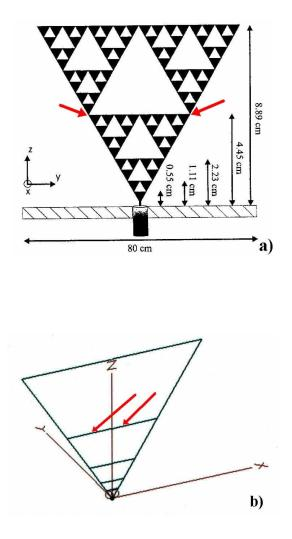
Figure 6 Serpinski monopole antenna, upper figure, and an equivalent wire model lower figure.
