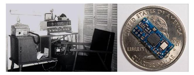
Figure 2. Left: vintage Ham radio transmitter/receiver setup. Right: a wireless sensing node comprising a 900MHz transceiver, low power microcontroller, and non-volatile memory.
