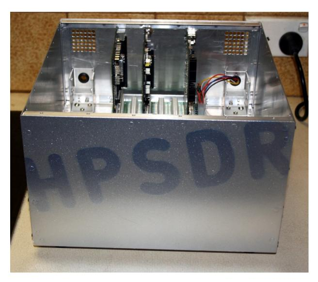
Figure 6 VK6VZ's partly-built HPSDR transceiver in VK6CG's prototype case.
