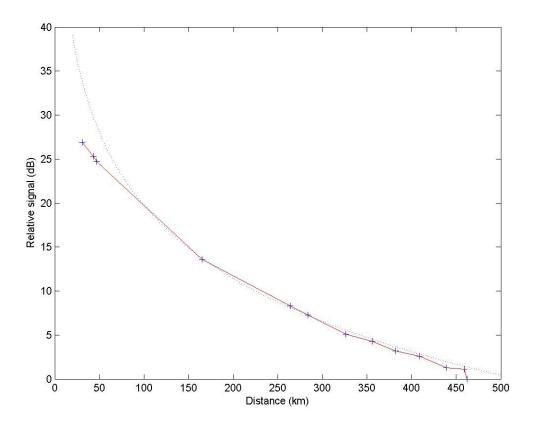
*Figure 8* Plot of signal strength vs. distance. The solid line is a plot of observed levels. The broken line is from Eqn. 10.
