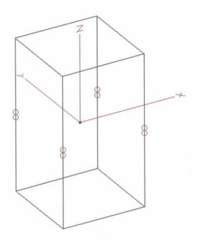
Figure 7 Multiple fed dipole antenna, wire model.
