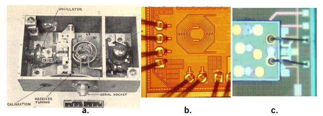
Figure 3. Evolution of RF design showing a.) Bulky vacuum-tube design using high quality passives, b.) Current RF design using on-chip passives, and c.) Our vision of future RF design using fast commodity transistors and high-quality passive devices
