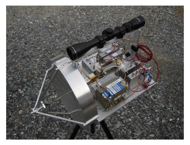
Figure 1 – Example of 241/322/403GHz portable Amateur Radio station
