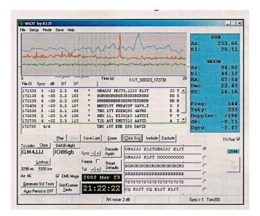
Figure 11 Main screen of WSJT in JT44 mode displays K1JT's EME contact with GM4JJJ. The large box shows WSJT's attempts to decode GM4JJJ' signal in successive 30-second periods.
