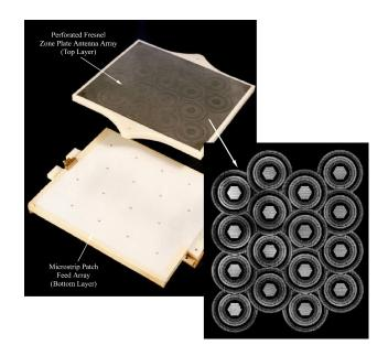
Figure 12. Array of perforated Fresnel zone plate antennas at 30 GHz.
