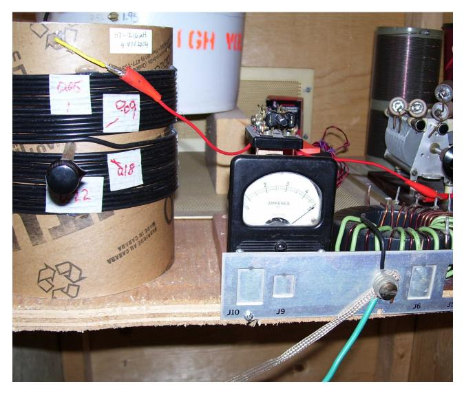
Figure 6 Aerial ammeter: just over 5 amperes to a 100 metre wire
