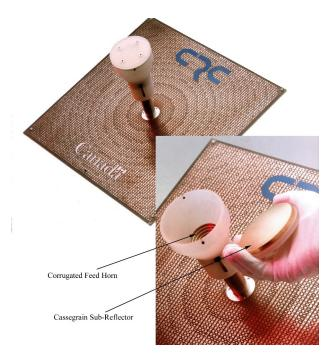
Figure 6. Dual-band (20/30 GHz) reflectarray with Cassegrain sub-reflector.
