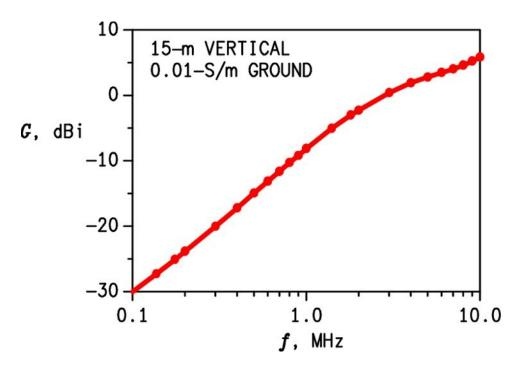
Figure 5. Low-angle/ground-wave gain of 15-m vertical antenna.
