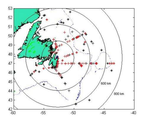
*Figure 9* Receptions of the 10 watt 187 kHz beacon. Red symbols indicate readable signals, black symbols indicate no signals heard. Note how a reception path over the ocean extends farther than those over the land.
