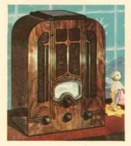
This six-tube superheterodyne has a tuning range from 540 to 18,000 kilocycles, covering long and short waves. The T6-1 is a table model in a lovely cabinet and the price is \$49.95.
