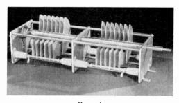
Figure 1. A high efficiency split-stator condenser for  $\mathbf{C}_4$  such as recommended by the author.
