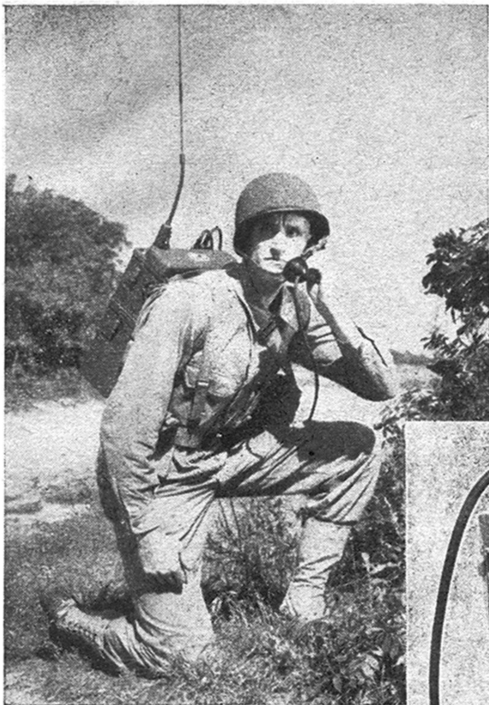
Both a headset and handset are used with the F.M. walkie-talkie so two can listen in. There are also two types of antennas
