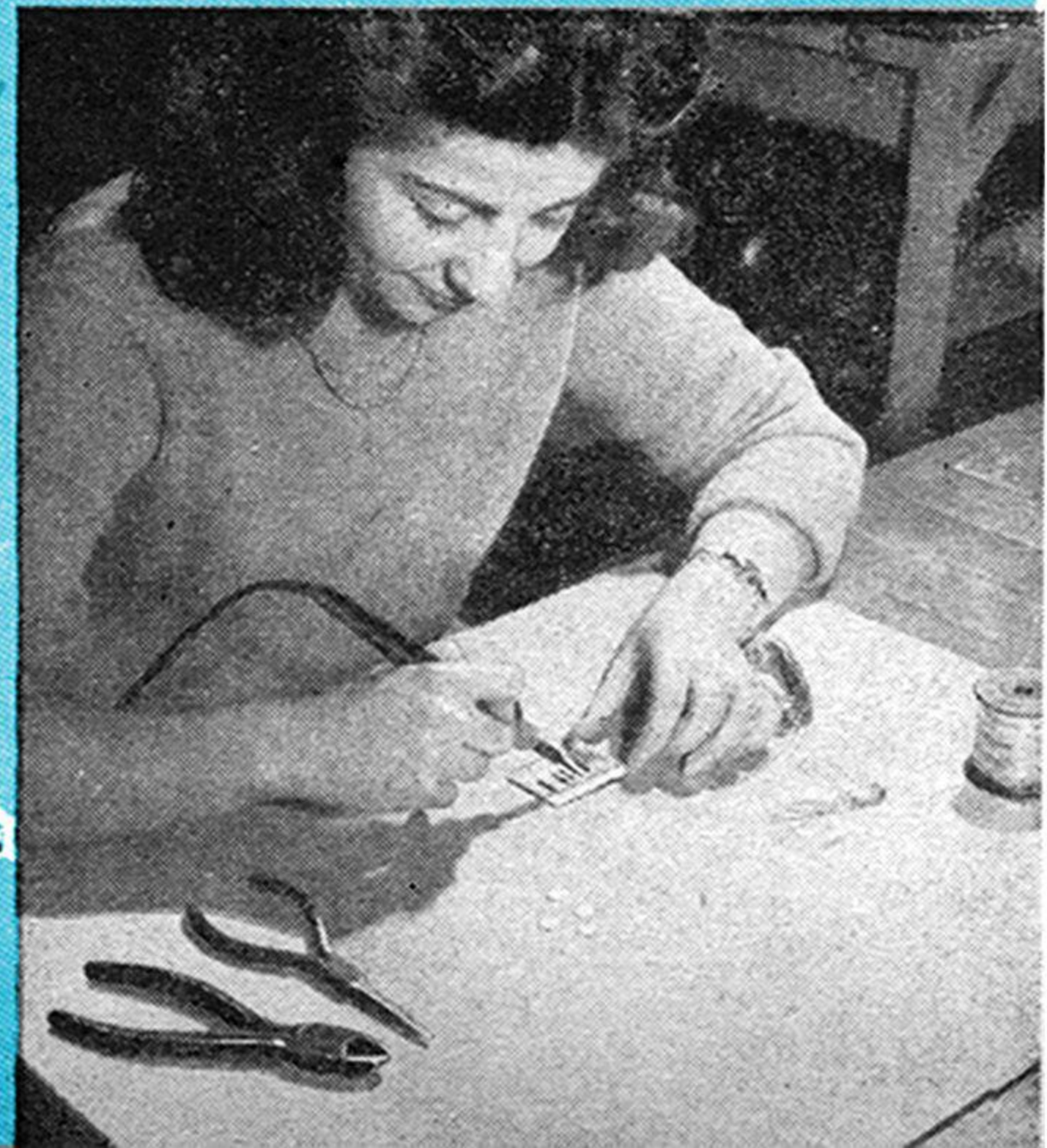
A small penlike soldering iron is used to fasten the miniature tube leads to the ceramic base plate.
