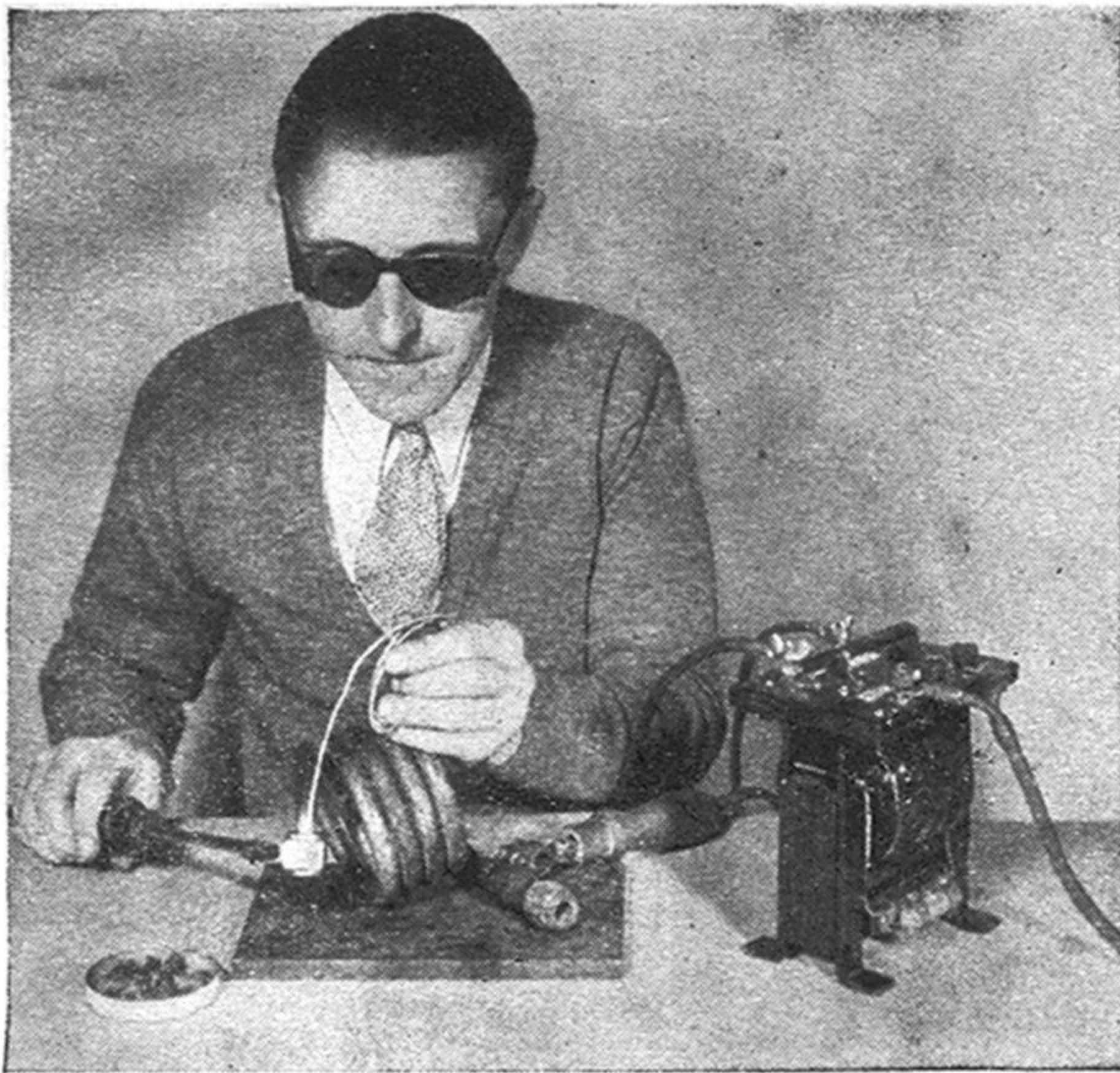
The white-hot carbon heats work enough to melt solder freely
