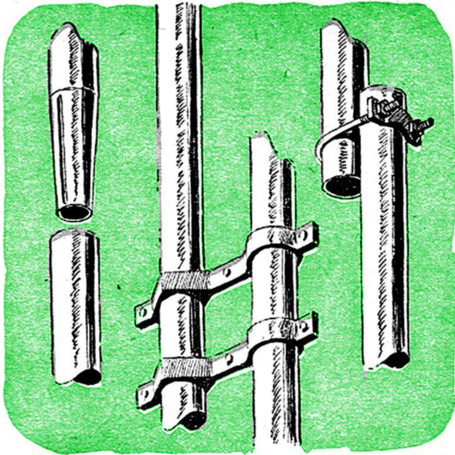
MAST CLAMPS. To gain height you can stack mast sections one above the other. Some types have nesting ends; others may be joined by clamps made to fit standard mast diameters.
