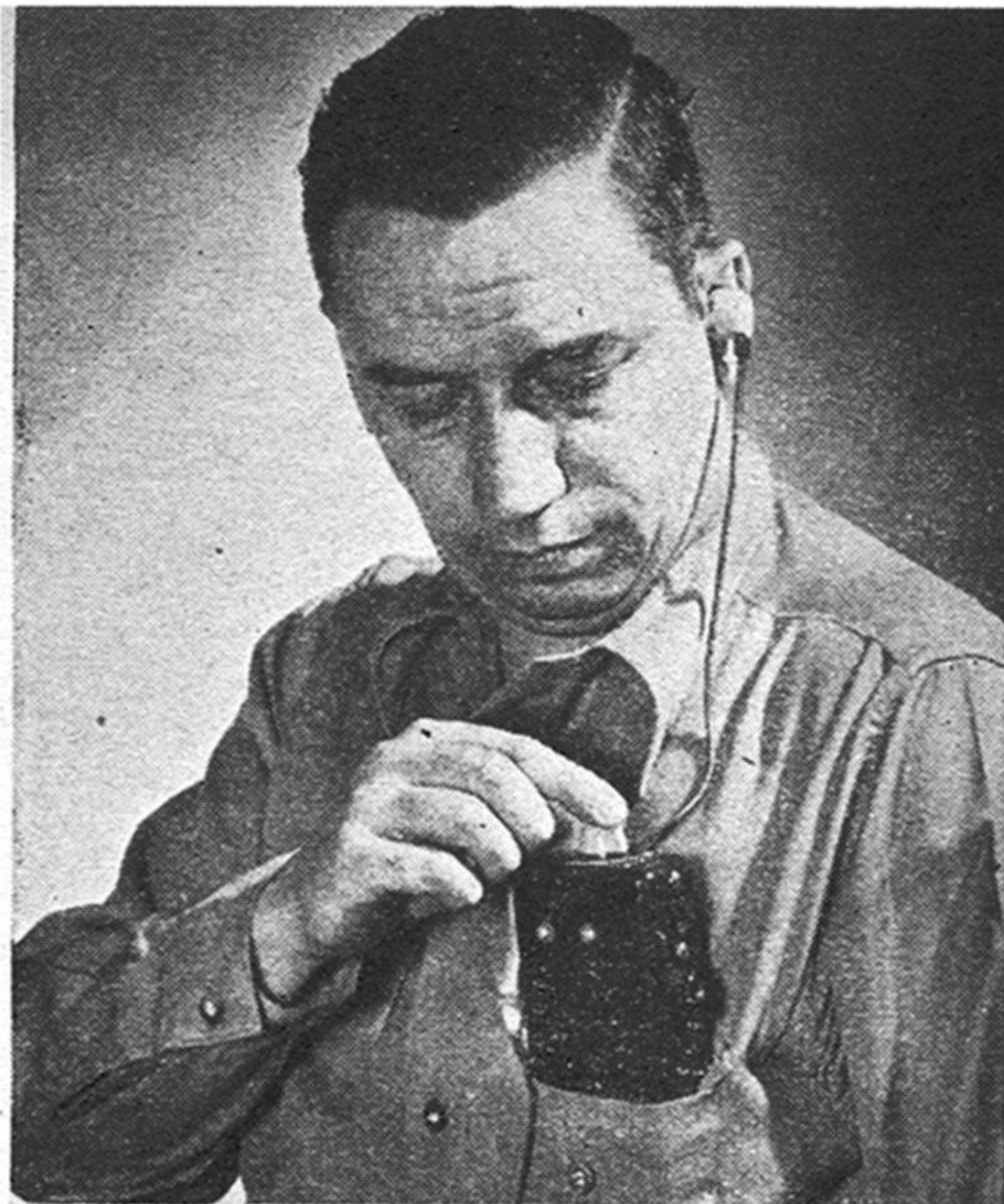
It's light as well as small. Complete with batteries, the set weighs less than 14 ounces.
