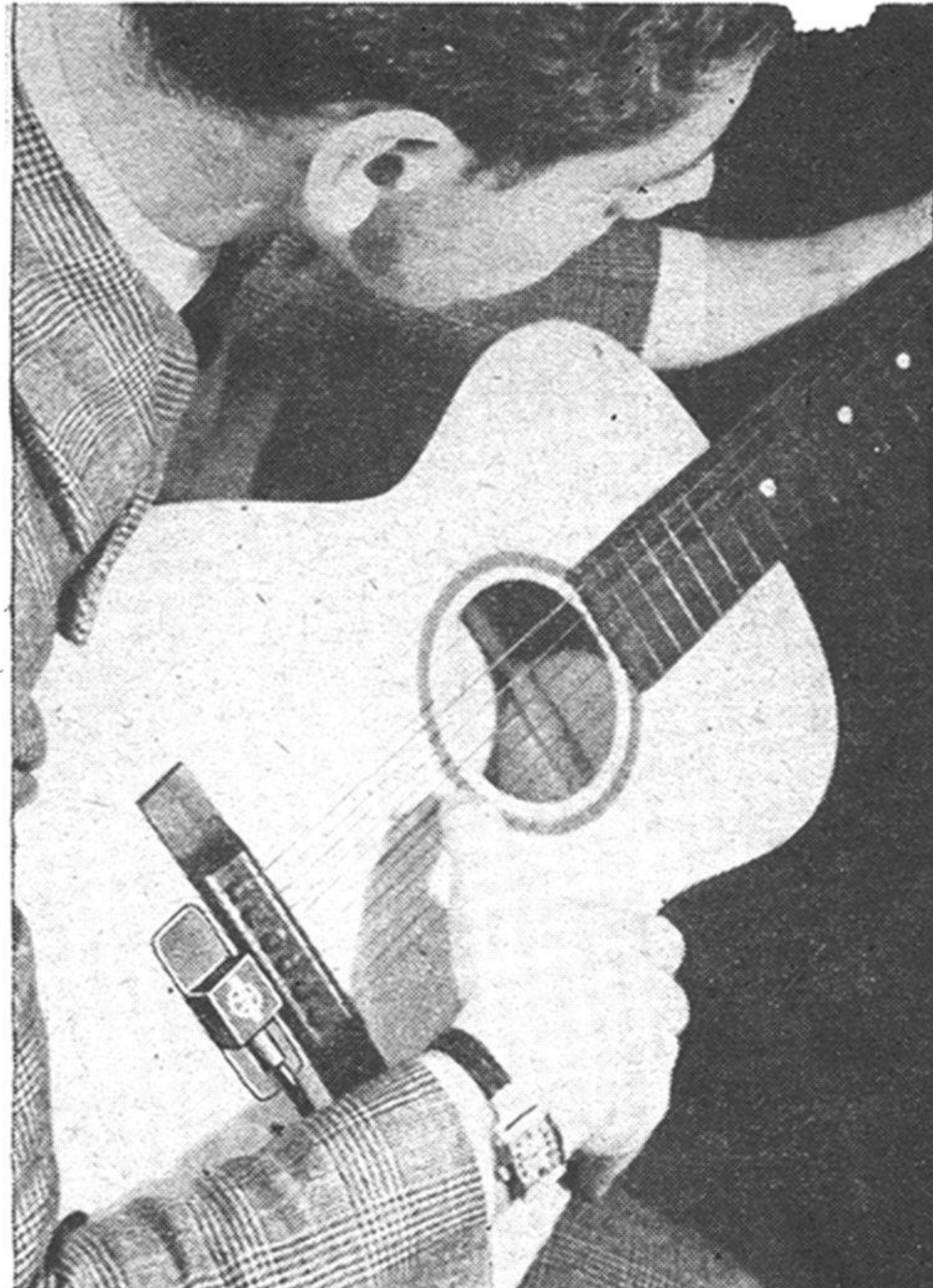
A little rubber cement was used to attach the contact microphone to this flat-top guitar. You can find the best place for the mike by actual trial.
