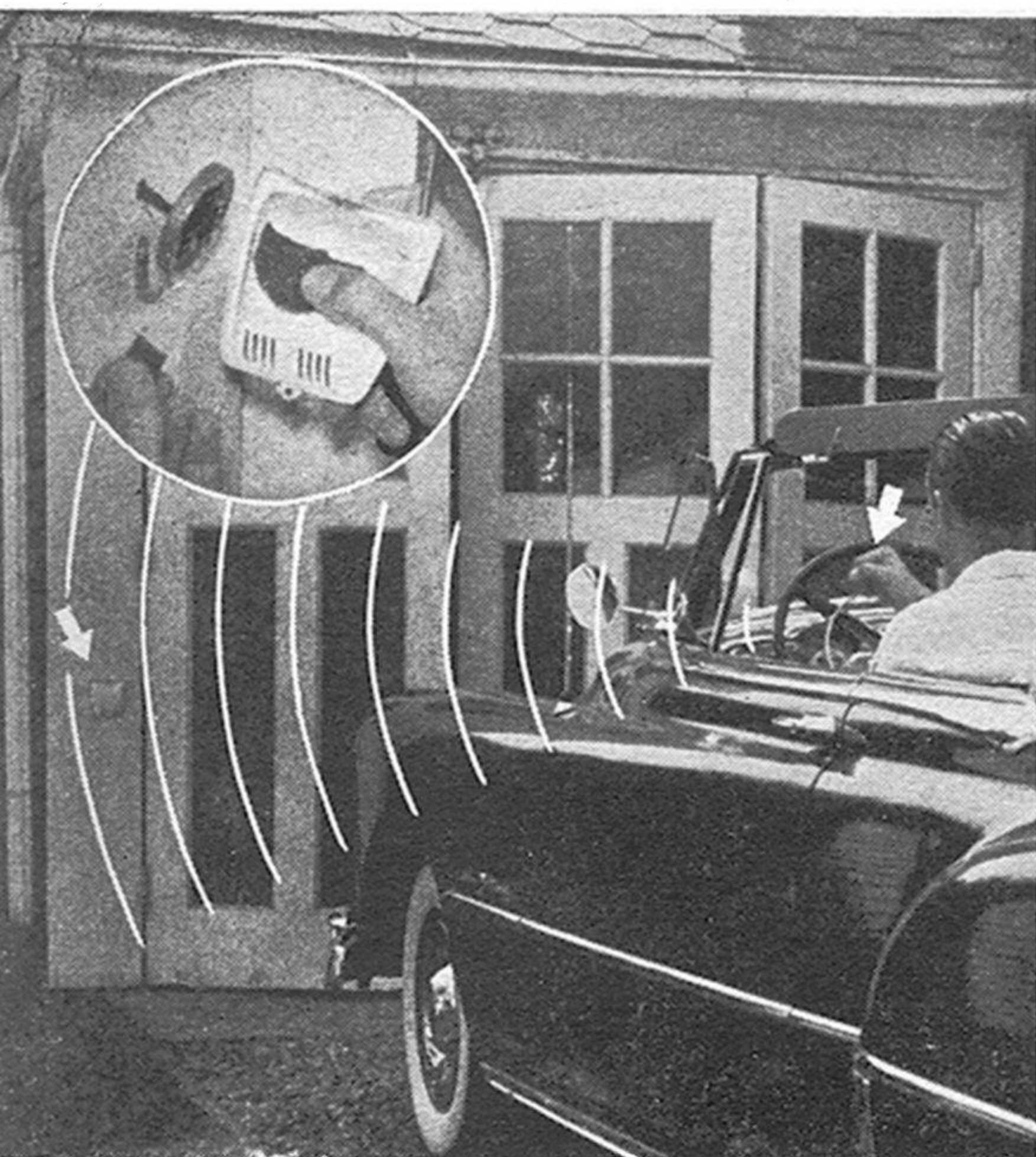
Automatic garage doors can be honked open with this sound-operated switch. Mike is cushioned on rubber, enclosed in a watertight hood.
