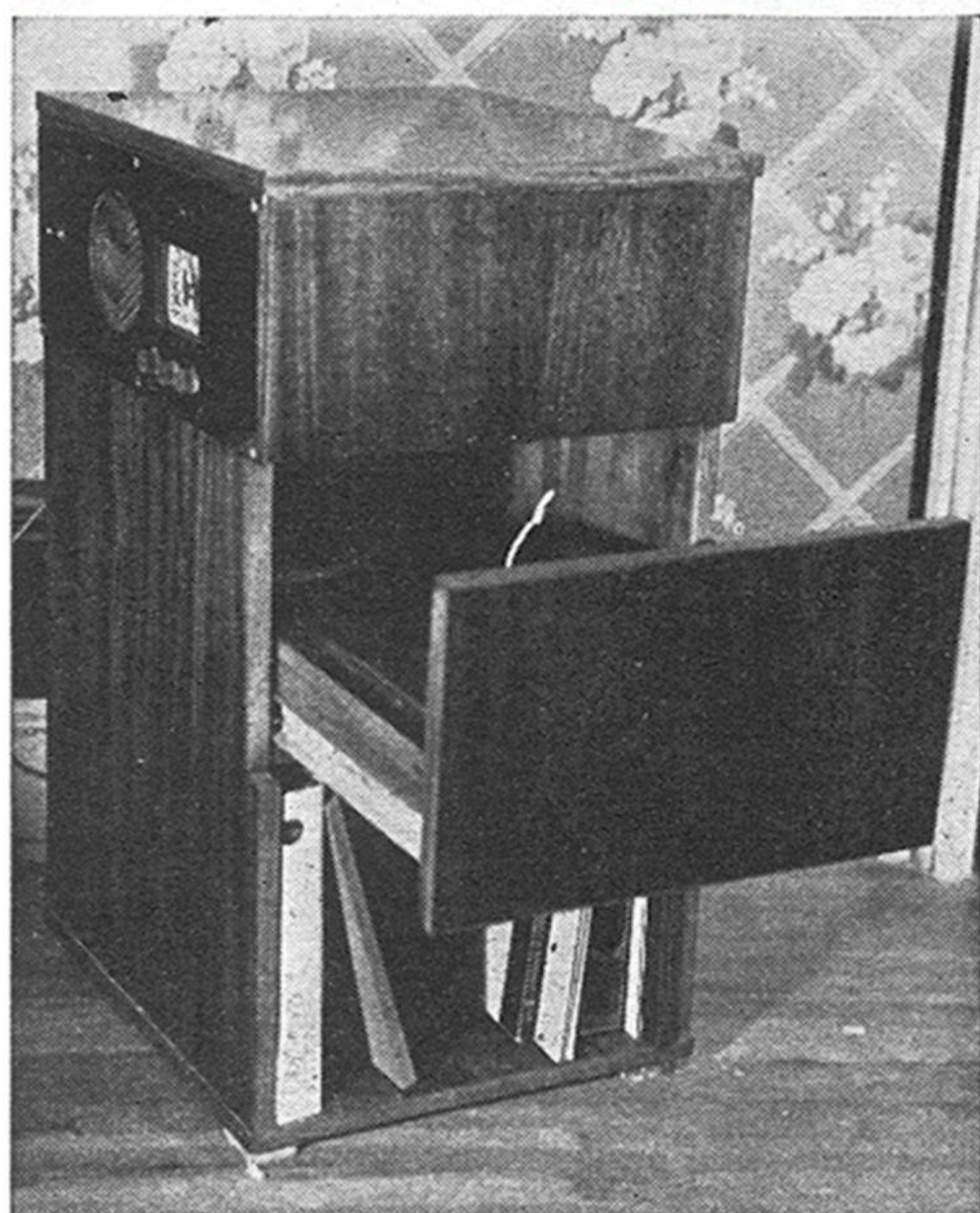
Finished cabinet has veneer strips on all exposed edges. Radio panel is piece of plastic.
