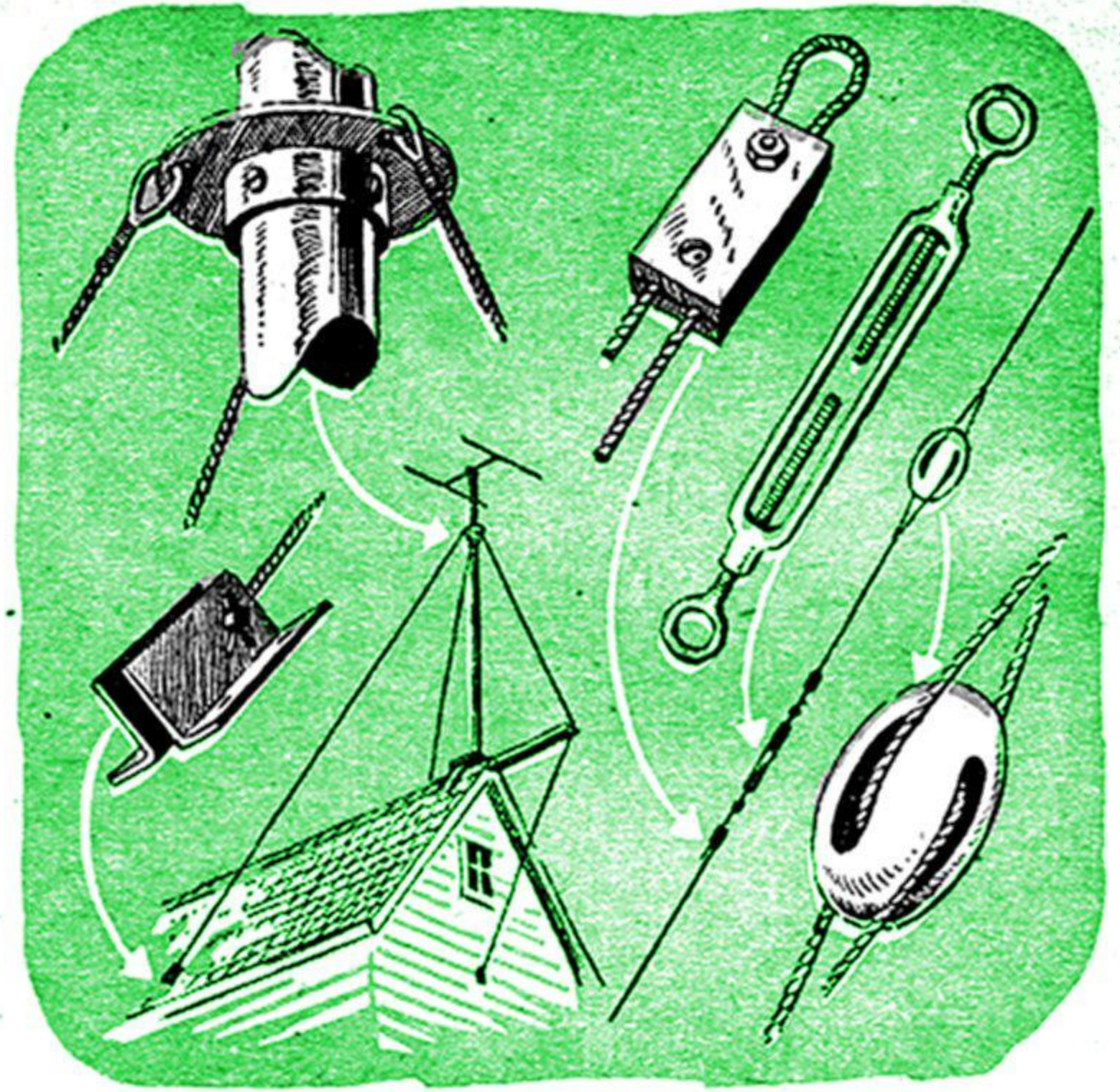
GUYS. Support high antennas with three or four equally spaced, firmly anchored guy wires. Build out extra anchor point on roof if needed. Use strain insulators to break long wires.
