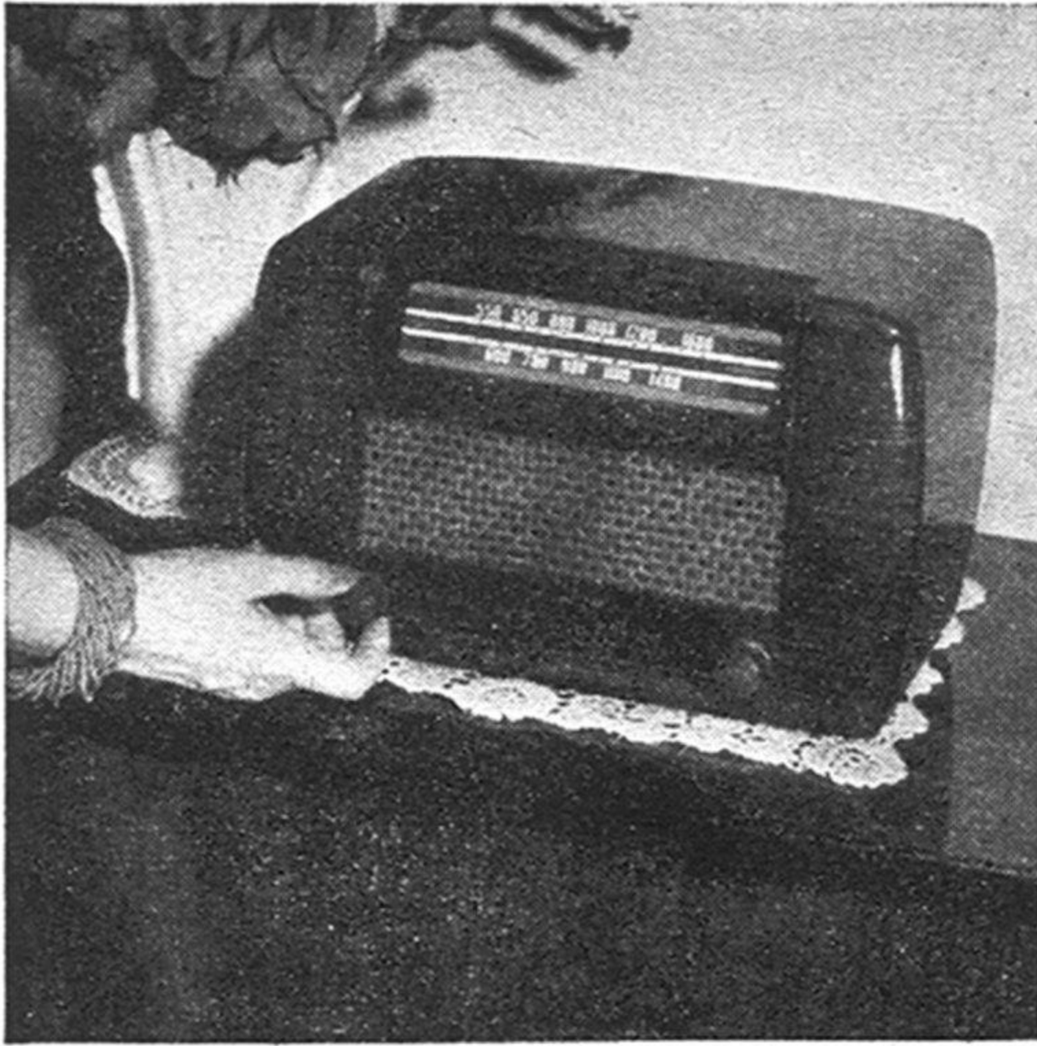
Two jacks and a toggle switch, installed on the chassis of a table radio as shown above, permit the small set to be connected to the speaker of a console model by wires leading from the jacks
