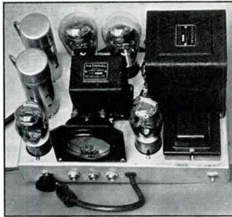
FIG. 66 — THE UNIT CONTAINS A CRYSTAL-MICROPHONE SPEECH AMPLIFIER, DRIVER AND CLASS-B MODULATOR, AS WELL AS A POWER SUPPLY FOR THE LOW-POWER STAGES
