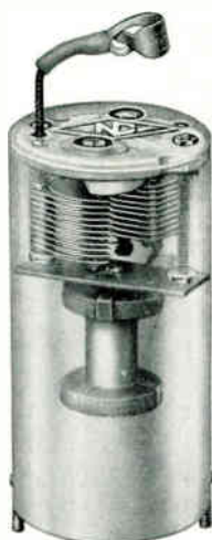
The improved model National Air Dielectric condenser-tuned I.F. transformer as used in the National FB7A, AGSX and HRO receivers
