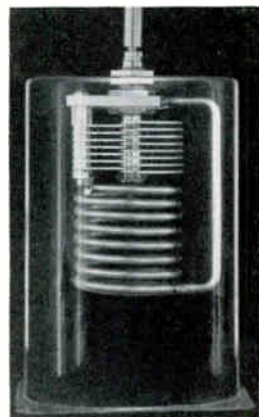
FIG. 5—AN "X-RAY" VIEW OF ONE OF THE BUFFER TANK CIRCUITS
