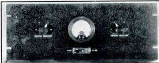
FIG. 10 — PANEL VIEW OF THE EXCITER UNIT, SHOWING THE TWO CRYSTAL SELECTOR CONTROLS (RIGHT AND LEFT), WITH THE BANDSWITCH BELOW THE PLATE MILLIAMMETER
