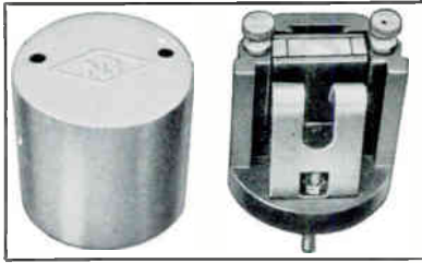
FIG. 18—THE NATIONAL TYPE CHT CRYSTAL HOLDER MAY ALSO BE USED WITH SPACER BARS AS HERE SHOWN TO PROVIDE AN AIR-GAP TYPE OF MOUNTING
