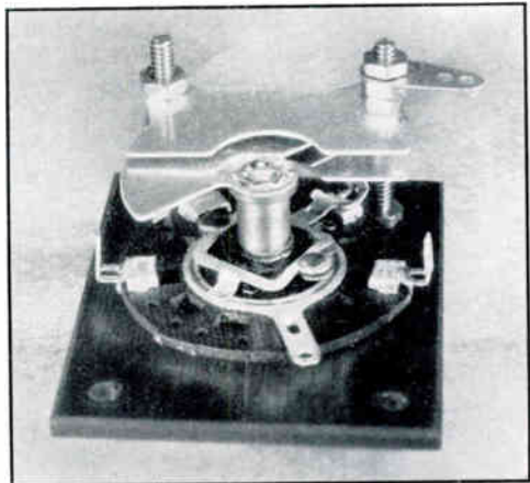
FIG. 9 — CLOSE-UP OF COMBINED CRYSTAL SELECTOR SWITCH AND OSCILLATOR TANK TRIMMER CONDENSER
