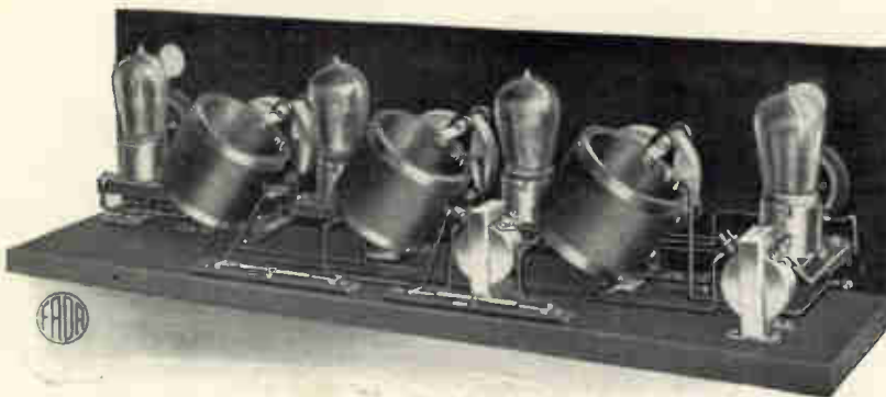
Rear view photograph of the four tube "Neutrodyne" receiving set. Note that the audio transformers are spaced well apart on the baseboard. This reduces the length of the wiring and reduces the capacity of the circuit.
