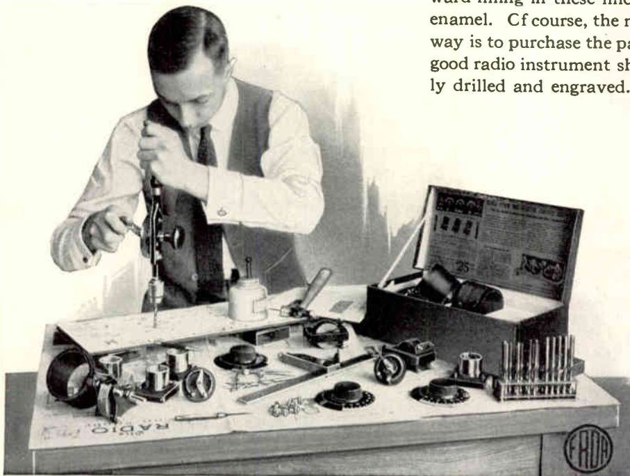
Showing a "Neutrodyne" receiver panel in the process of being drilled, using the paper template supplied with this book.
