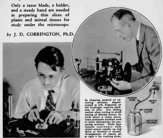
COULD you put a camel through the eye of a needle? Absurd, of course, yet it might be accomplished if one sliced up a camel on a microtome. This delicate precision instrument can cut sections of plant and animal structure so thin that the opening in a needle seems as wide as a barn door in comparison.
