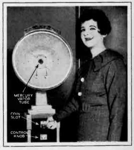
Powerful violet ray lamp machine being installed in New York City shops delivers sun tan for seven minutes when coin is inserted. Sun-bathers sit on chair in front of device.
