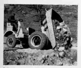
Backward-running dump truck lets driver run up to pit or fill without craning neck. This model carries 6-ton loads.
