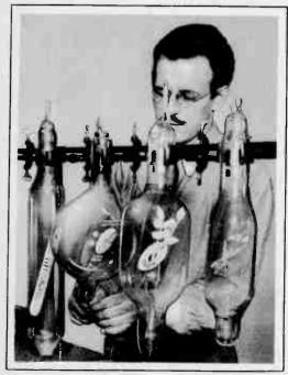
Advertising emblems sealed into these cathode ray tubes glow weirdly under electron bombardment. Gilbert T. Schmidling (pictured above) builds these tubes for store window display. High voltage transformers are needed here.
