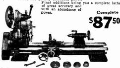
Back-geared: screw-cutting; automatic, reversible feeds. Sixteen speeds from 28 to 2,072 R. P. M. Cuts 4 to 72 threads per inch. Will ido ANY job within its capacity accurately and easily. TWO WEEKS TRIAL, money-back guarantee. Easy terms, Full line of attachments at reduced prices.
