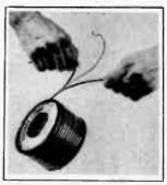
Cotton tape between wires of new rubber lamp cord permits separation of wires in "zipper" fashion.
