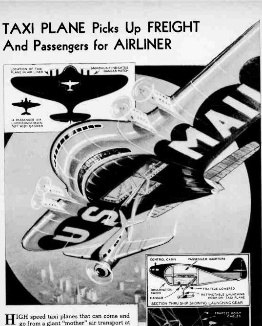
HIGH speed taxi planes that can come and go from a giant "mother" air transport at will are proposed as a means of providing fast, non-stop transcontinental air service. The smaller ship, released over a city, would land at the airport to discharge and take on passengers and freight, then soar upwards again to catch up with the slower airliner.
