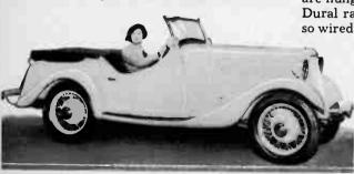
A de-luxe British Ford roadster containing a four cylinder motor which develops ten horsepower—one-eighth the power of the American Ford.
