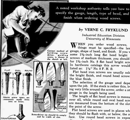
Holes for flat and oval head screws are countersunk to
