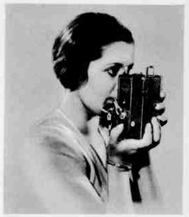
Combined home movie camera and projector has built in batteries which will operate film motor long enough to shoot 50 reels. When projecting, battery supplies power to bulb.
