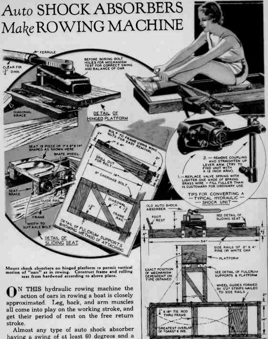
Heavier types of absorbers are best suited for rowing machine. Overhaul as indicated in sketches, then mount.
