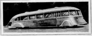
The new streamlined bus is the latest in aerodynamic design with a rear mounted motor to avoid obnoxious engine odors in passenger compartment.
