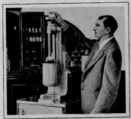
Demonstrating the quick action freezer. The liquid is poured in and sprayed on cold cylinder walls to freeze in 40 seconds. It is then shaved off with a cutter knife.
