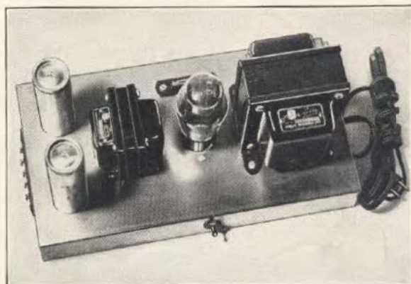
Top view of low voltage power supply. This will work with all transmitters requiring around 400 volts.
