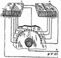
that the purpose of the dead contacts is to prevent short circuiting the cells of the battery in case the switch is left
