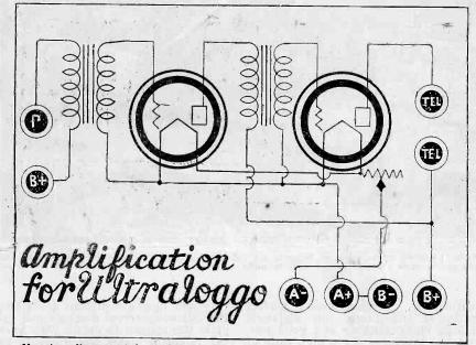
Here is a diagram of the amplifier which we recommend for use with the Ultrologgo Reflex. The combination will yield tremendous volume and the builder should be sure that his audio transformers are of the lowest available ratio.
