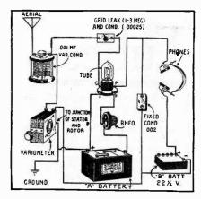
one-half of the total inductance of the variometer tunes the antenna circuit. Therefore, this instrument should be of quite a large size.
