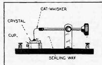
will hold the cat's whisker on it. Jars and jolts will not affect it. You will have, to all purposes, a fixed crystal, but one which easily can be adjusted by removing the wax and reapplying.
