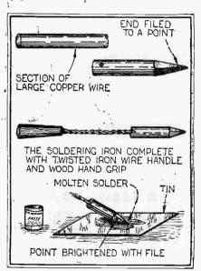
1 or No. 0 copper wire. The end is pointed with a file as shown in the accompanying illustration. A hole is drilled in one end through which is twisted a wire as per sketch, this to be driven or screwed into a wooden handle. This iron may be brought to a working heat in a small alcohol flame. It will retain its heat for a fairly long time.
