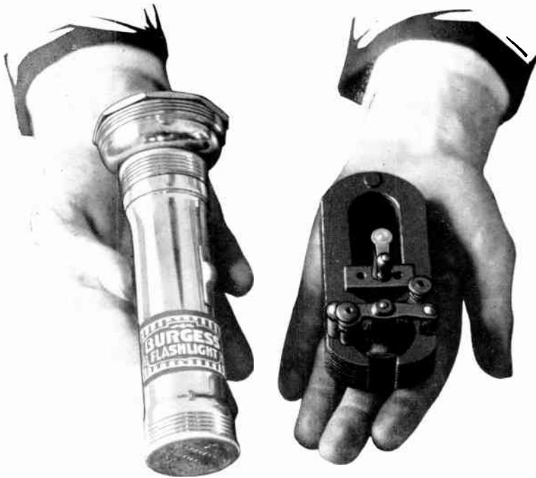
FIG. X. THE FLASHLIGHT AND HANDGENERATOR SHOWN HERE EACH DELIVER MORE POWER IN NORMAL OPERATION THAN THAT TAKEN BY THE TRANSMITTER WHEN WORKING SEVERAL HUNDRED MILES
