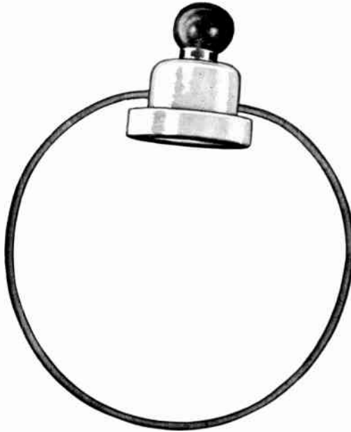
FIG. VIII. A 2- \frac{1}{2} VOLT FLASHLIGHT BULB HAVING A 3 INCH DIAMETER LOOP OF INSULATED WIRE CONNECTED TO ITS TERMINALS WILL INDICATE IF THE TRANSMITTER IS OSCILLATING PROPERLY WHEN THE LOOP IS BROUGHT NEAR THE COILS OF THE TRANSMITTER THE LAMP FILAMENT WILL GLOW
