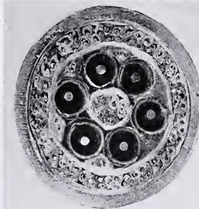
CROSS SECTION of a six-coaxial cable (left) shows position of coaxials with respect to regular telephone wires. Fanned-out view of cable at right shows construction of conductors in the one sheath. Width of waveband carried depends on amplifying equipment, not on cable.
