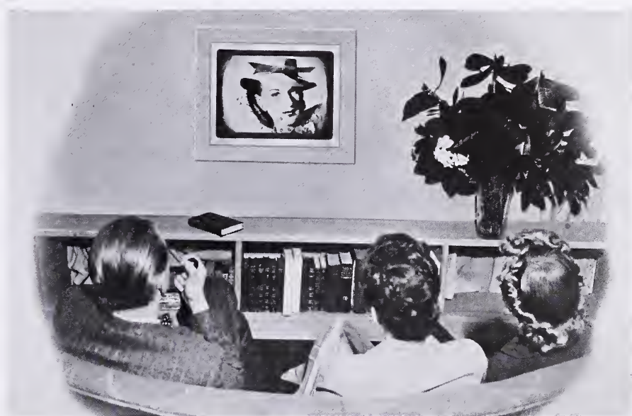
BUILT-IN TELESET—The mechanism is concealed, leaving an 18-inch "direct view" screen visible. A "direct view" picture, as distinguished from reflective and projection systems, is shown on the flattened, luminescent screen-face of a large picture receiving (cathode-ray) tube.
