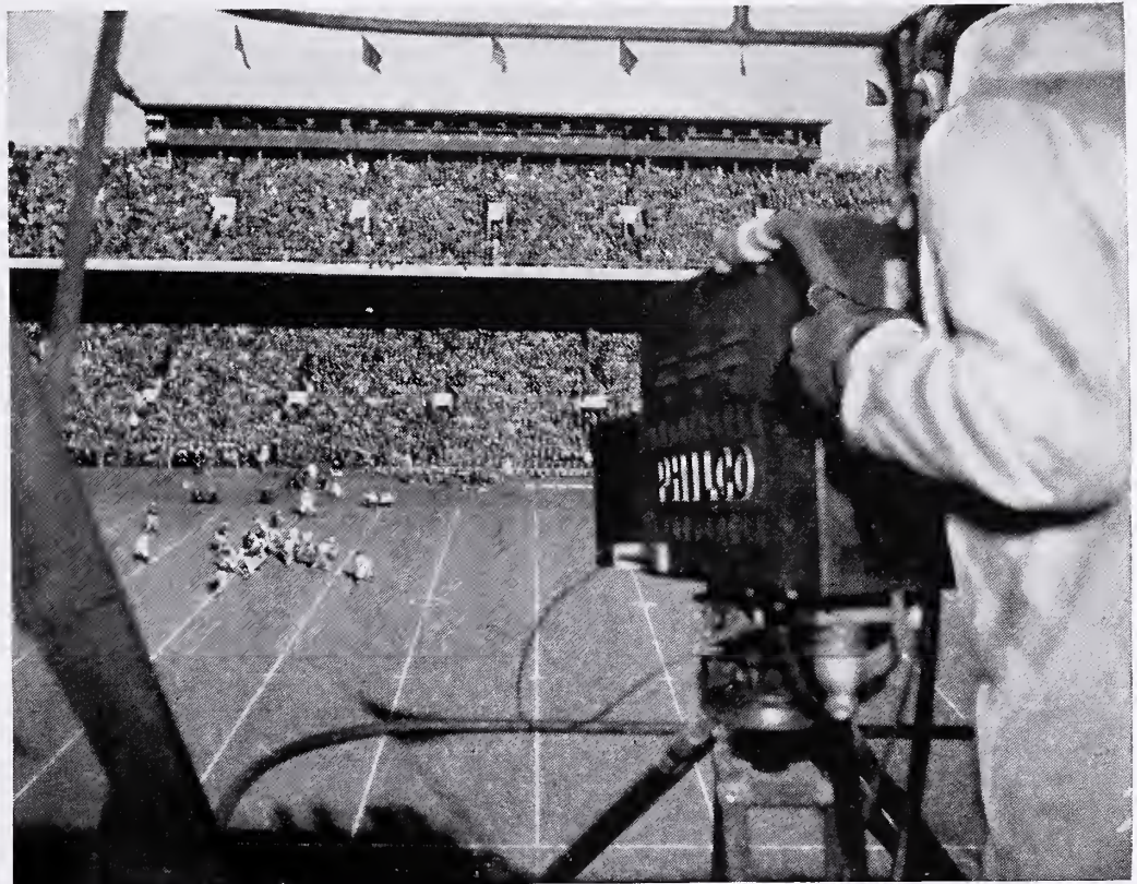
One of the two television cameras placed high above the 50-yard line, on specially-built platforms near the top of the South Stands. One camera has a wide lens for remote pick-up; the other is equipped with a telephoto lens for close-up pictures.
