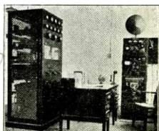
TRANSMITTER 1000 WATTS
