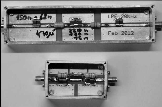
Fig 35: The two versions of the lowpass filter that were built.
