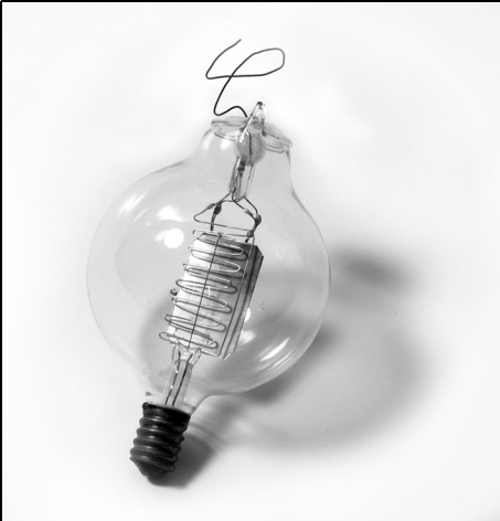
Fig 2: The Deforest long plate audion.
