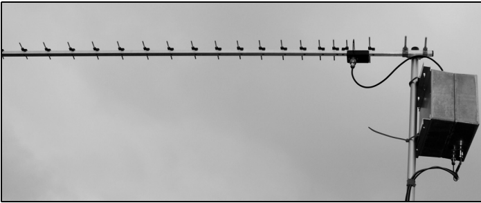
Fig 7: Transverter mounted on it's mast with the 19 element 23cm Yagi.
