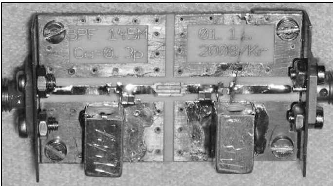
Fig 15. The simulation converted into a prototype with SMA connectors. The circuit must now be measured on the network analyser.
