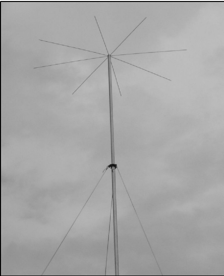
Fig. 2: The top load made from thin aluminium rods is only visible in the close-up photograph.
