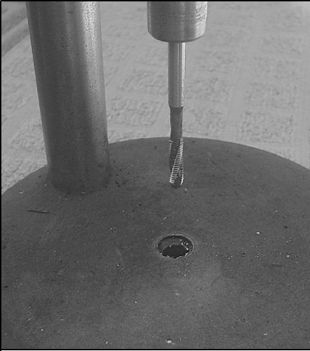
Fig 3: A spiral flute machine tap for tapping tough materials
