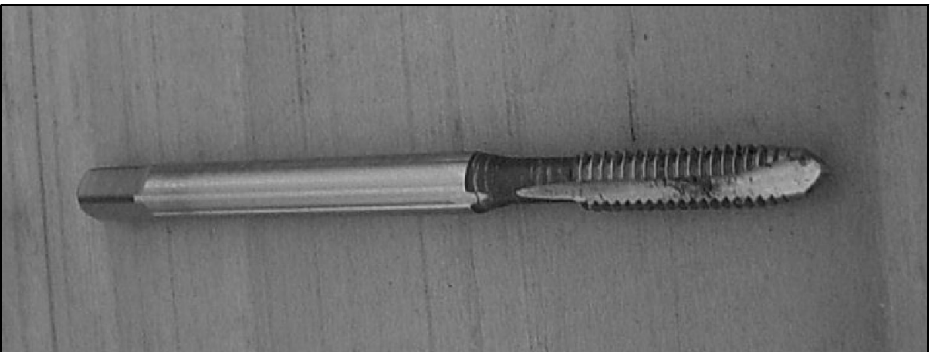
Fig 2: A typical machine tap with the spiral tip.
