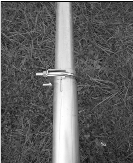
Fig. 6: The individual tubes are fitted into one another and secured with clips.
