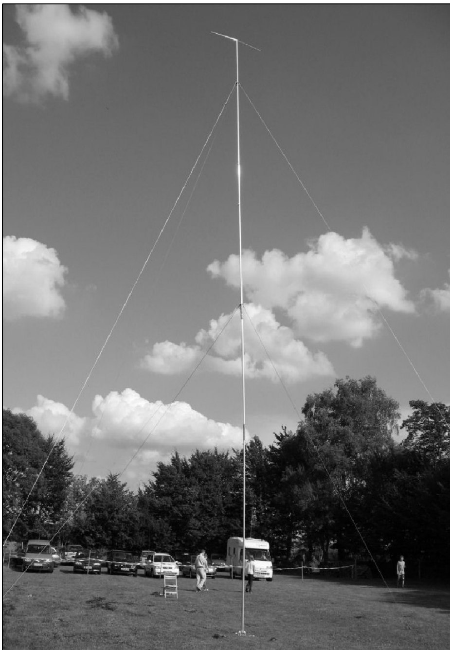
Fig. 1: Top loaded \lambda/4 vertical antenna for 80m on field day for the Itzehoe club (MØ5).
