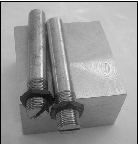
Fig 14: Filter block machined to size ready for drilling and two resonator rods with slotted ends and lock nuts.
