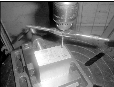
Fig 13: Using a tap wrench to start the threads guided by the tap held in the drill chuck.
