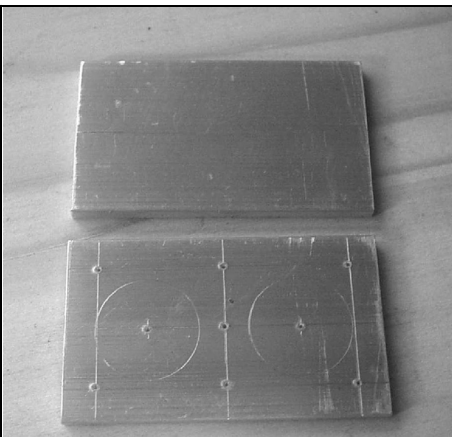
Fig 10: Top and bottom covers cut to size and top cover marked out and centre punched for drilling. The bores have also been marked to ensure the cover fixing holes do not intrude on the bores.
