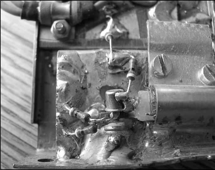
Fig 3: Detailed view of the transistor in the coax cable pulse generator.
