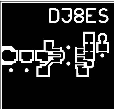
Fig 8: PCB layout of the measuring head.
