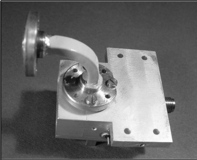
Fig 2: Rear view of module 1 showing waveguide output.
