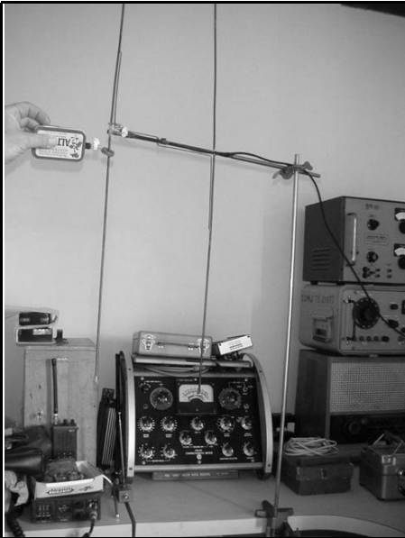
Fig 4: Signal Detector measuring current in an HB9CV antenna.
