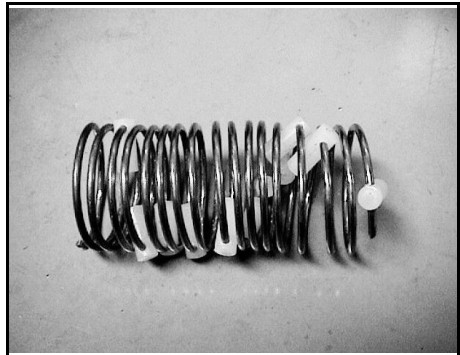
Fig 4: Fitting spacers onto wound helix.
