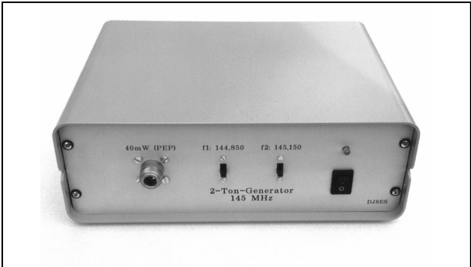
Fig. 1: 2-tone generator for the 2m band, ready for operation in a housing.
