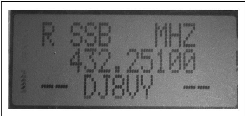
Fig 2 : Example of 3 line display.
