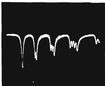
Fig.9: Principal and Spurious Resonances at 9th Overtone; (a) without compensation; (b) with compensation Y: 5dB/div; X: 20 kHz/div
