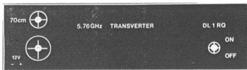
Fig.1.1 Front panel for DL1RQ NT6-1: 145 x 40mm Material: Epoxy PCB 1.5mm thick, copper-clad both sides
