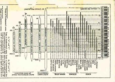
Chart prepared by the Stromberg-Carlson range of the various types of receivers Acoustical Lab tories showing tonal
