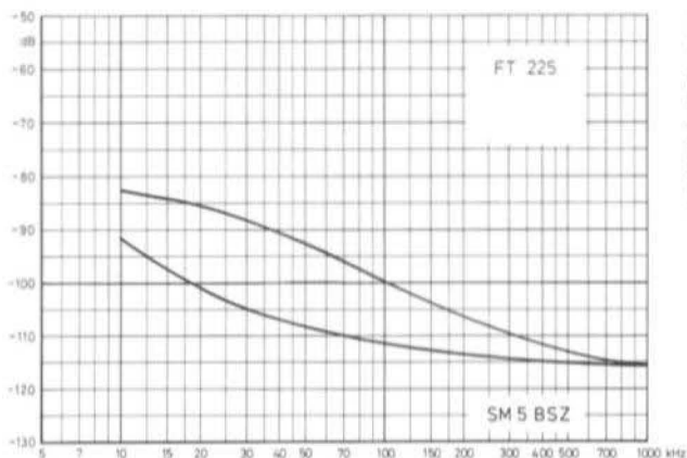
Fig. 1: Vertical scale = power difference to the main carrier; Horizontal scale = frequency difference to the carrier. Noise sidebands from the FT 225 before (above) and after (below) modification
