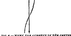
FIG. 5 - WHEN THE CURRENT IN THE CENTER OF THE RADIATOR IS ASSUMED IN THIS PARTICULAR CASE, THE CURRENT DISTRIBUTION IS SHOWN.
