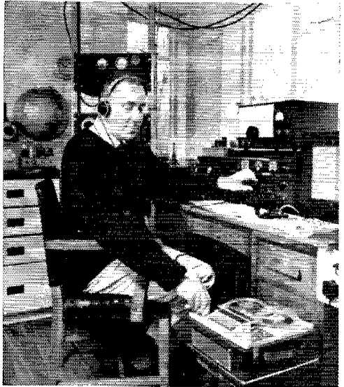
G6AG's station consists of a 1-kw. transmitter, crystal-controlled converter and home-constructed receiver, and a 8 over 8 Yagi antenna 50 feet high.
