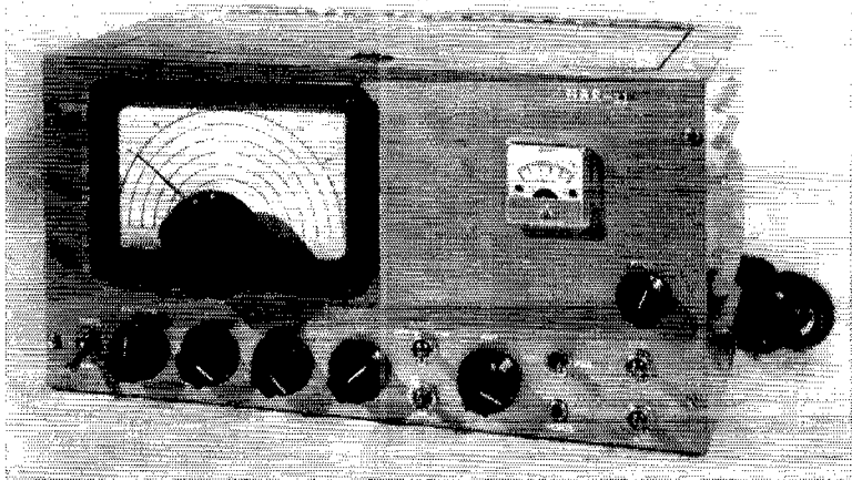
Fig. 1—Panel layout of the HBR-11. Controls along the bottom are the send-receive switch, S_1 , antenna trimmer, C_{11} r.f. gain, R_1 , mixer gain, R_2 , i.f. gain, R_3 , a.g.c. switch (above), S_4 , calibration oscillator switch (below), S_2 , audio gain R_4 , phones/speaker switch, S_5 , phone jack, J_1 , and in the column of three at the right, b.f.o. tuning, top, C_{12} , b.f.o. switch, S_6 , and a.c. power switch, S_3 .
