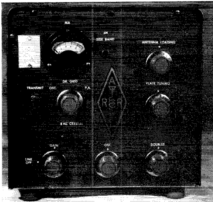
Fig. 1—The cabinet and the 9 × 10-inch panel are homemade. The meter switch is below the meter. Along the bottom are the audio gain control and tuning controls for the oscillator and doubler. The antenna-loading and amplifier-tuning controls are at the upper right. The switch to the left of the meter switch actuates an antenna relay.
