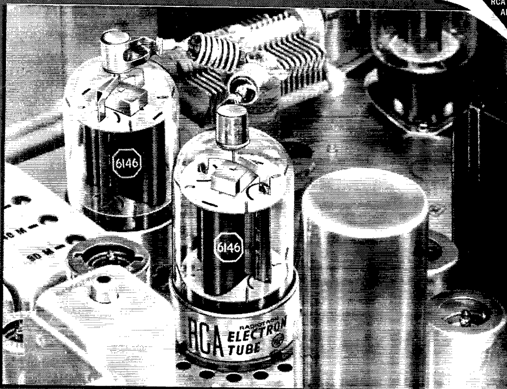
Inside view of the HT-37, showing the two RCA-6146's in parallel in the linear final.
