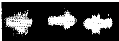
50-Mc. pulses from ZE2JV, recorded when flutter was relatively severe and beam tests showed a high degree of scatter.
