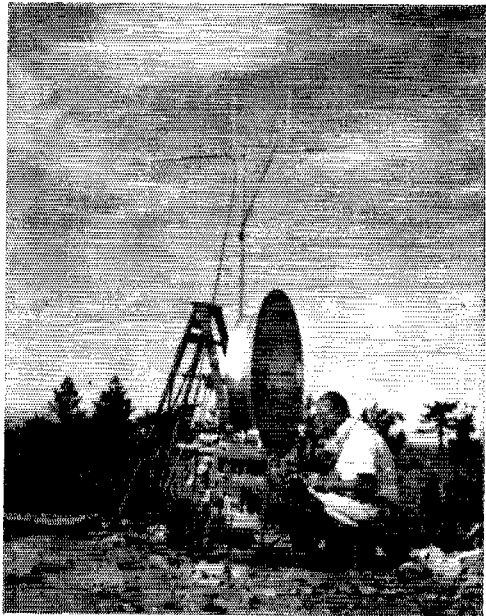
The southern end of the 225-mile 1296-Mc. record reported in September QST. Russ Robertson, W6DQJ, 6, operating atop Mt. Pinos, is shown as he worked W6MMU-6 on Mt. Hamilton. Equipment was crystal controlled, both transmitting and receiving, and operation was by c.w. only. The path is obstructed at three points.
