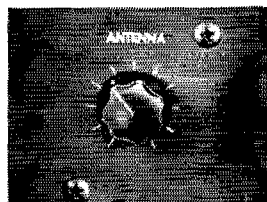
Antenna trimmer for optimum antenna matching.
