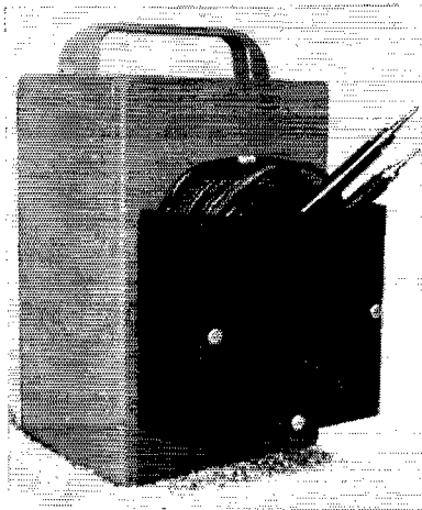
Fig. 1 — A utility box can be used to good advantage as the storage bin for V.T.V.M. test leads as shown in this assembly.
