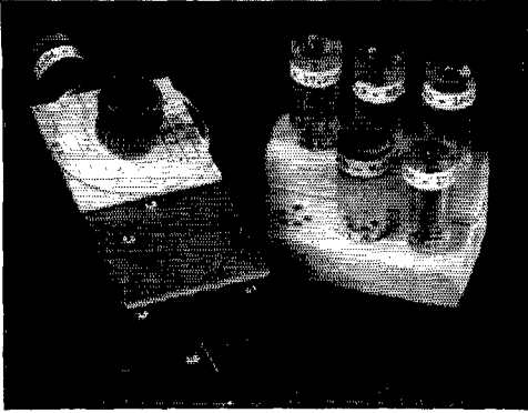
Fig. 21-20 — A compact and light-weight grid-dip meter for one-hand operation.
