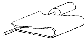
Fig. 2—A heat-dissipating clip as described in the text.
