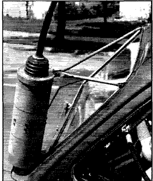
Base-loading coil for frequency adjustment, and method of mechanical bracing to the car. The coil, a surplus roller-type variable inductance, is inside a weatherproof cover made from phenolic tubing. It can be adjusted from the front seat of the car by means of a flexible shaft. The antenna in this installation extends ten feet above the coil and is topped by a capacity hat two feet in diameter.
